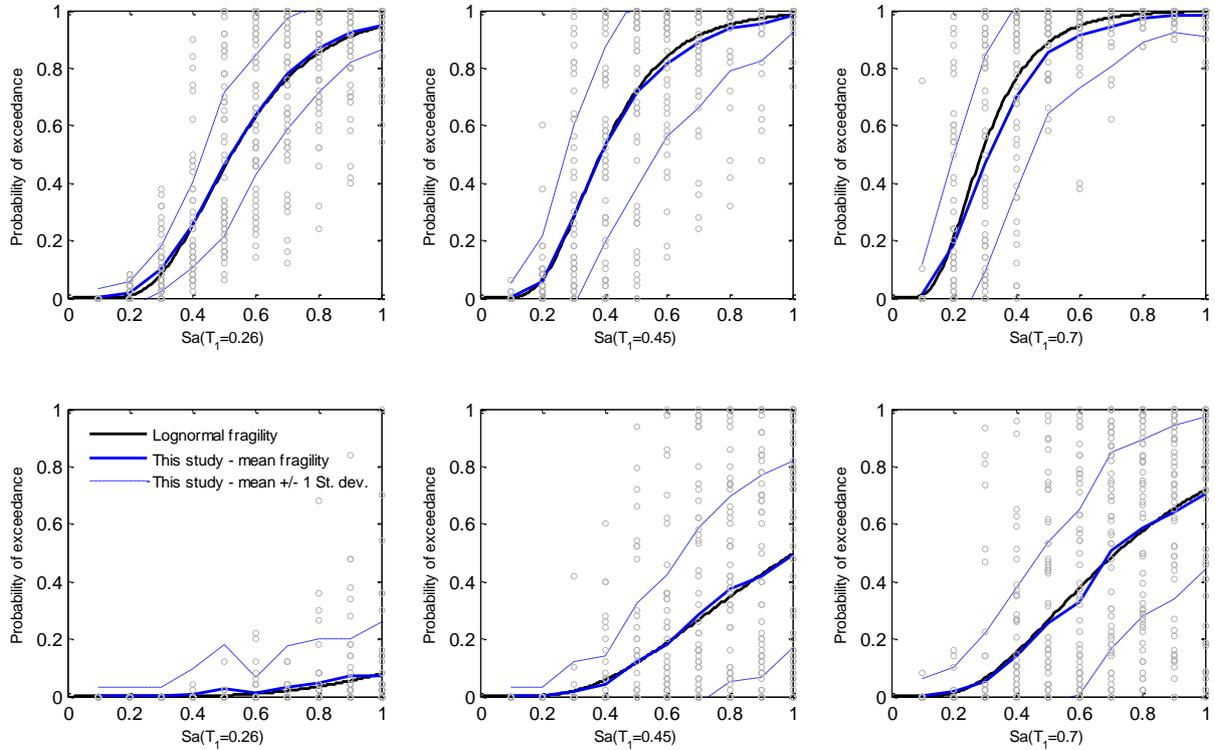
Figure 8. Mean, 16% and 84% percentiles of exceedance probabilities as a function of  $Sa(T_1)$ ; limit states of  $SD$  (upper) and  $Col$  (lower); 5 story buildings.
