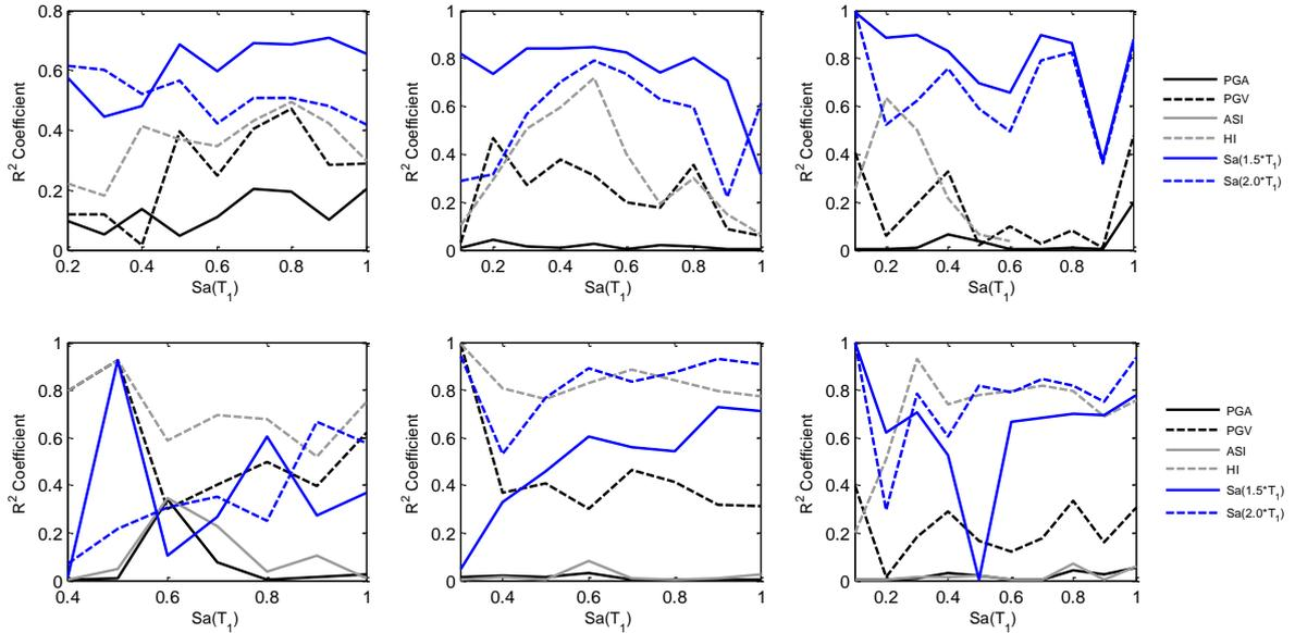
Figure 6.  $R^2$  regression coefficient for *PGA*, *PGV*, *ASI*, *HI*,  $Sa(1.50 \cdot T_1)$  and  $Sa(2.0 \cdot T_1)$  for limit states of *MD* and *Col*; 2 (left), 5 (middle) and 8(right) story frames.
