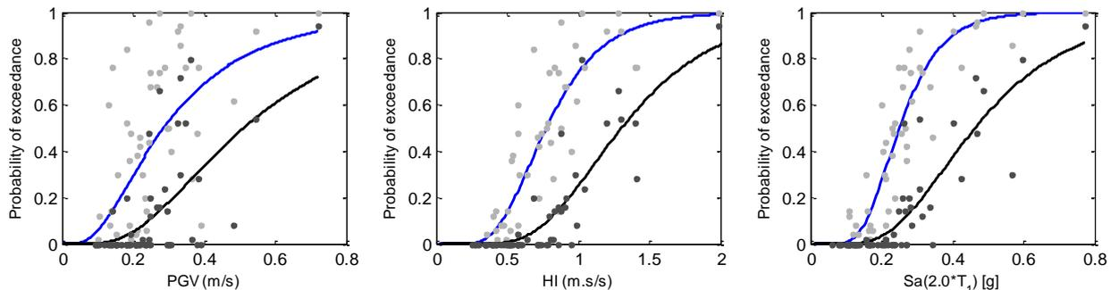
Figure 4. Lognormal fragility functions for 5 story frames -  $f_{LSi|IM_i,IM_j}(im_i, im_j)$ ; conditioned on  $Sa(T_1)=0.50$ ; limit states of  $MD$  (blue) and  $Col$  (black).
