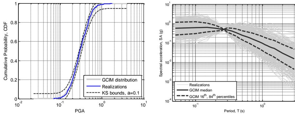
Figure 2. Target distributions and selected record sets for two story frames (PGA and spectral accelerations) conditioned on  $Sa(T_1)=0.5g$ .
