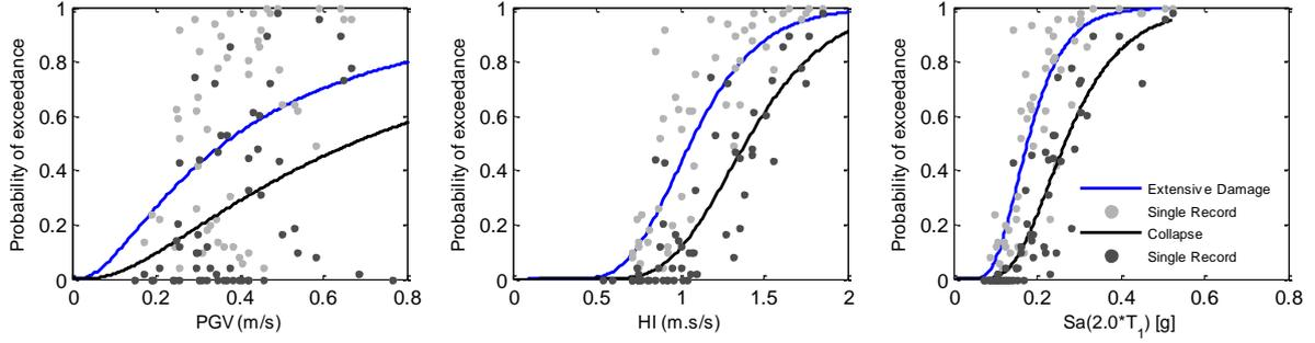
Figure 5. Lognormal fragility functions for 5 and 8 story frames -  $f_{LSi|IM_i,IM_j}(im_i, im_j)$ ; conditioned on  $Sa(T_1)=0.50g$ ; limit states of *MD* (blue) and *Col* (black).
