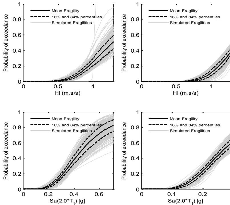
Figure 7. Individual, mean, 16% and 84% percentile fragilities -  $f_{LSi|IM,IMj}(im_i, im_j)$  - for intensity measures of  $HI$  and  $Sa(2.0*T_1)$  - limit state of  $Col$  - conditioned on  $Sa(T_1)=0.5g$ ; 5(left) and 8(right) story buildings.
