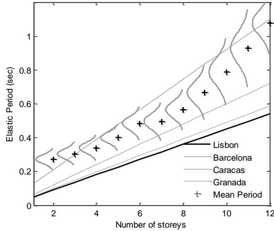
Figure 1. Sampled elastic periods of vibration of pre-code infilled frames and comparison with existing prediction for European cities.
