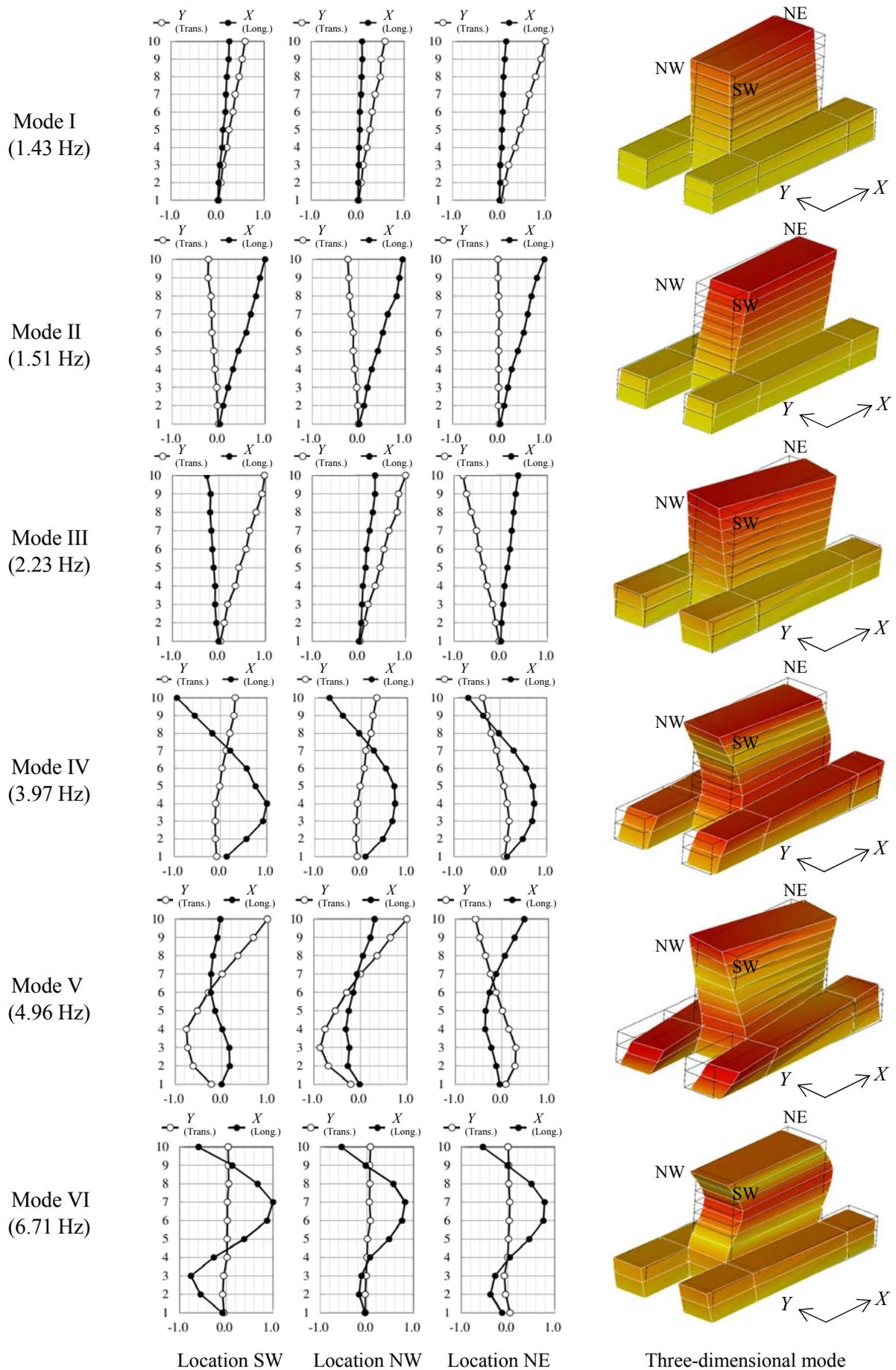
Figure 6. Identified modes at three locations (SW, NW, NE) and three-dimensional mode
