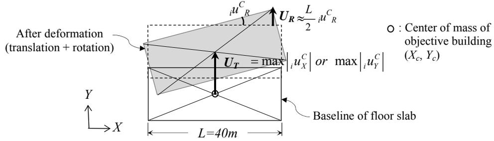
Figure 7. Illustration of plane vibration model (e.g. vibration in Y-direction)
