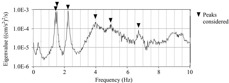
Figure 5. Eigenvalues of PSD matrix of response
