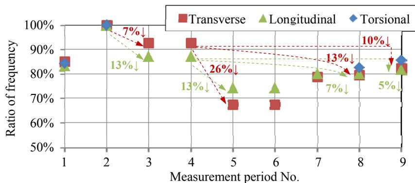
Figure 9. Changes in natural frequency based on ambient vibration measurements (represented by percentage based on measurement period No. 2)
