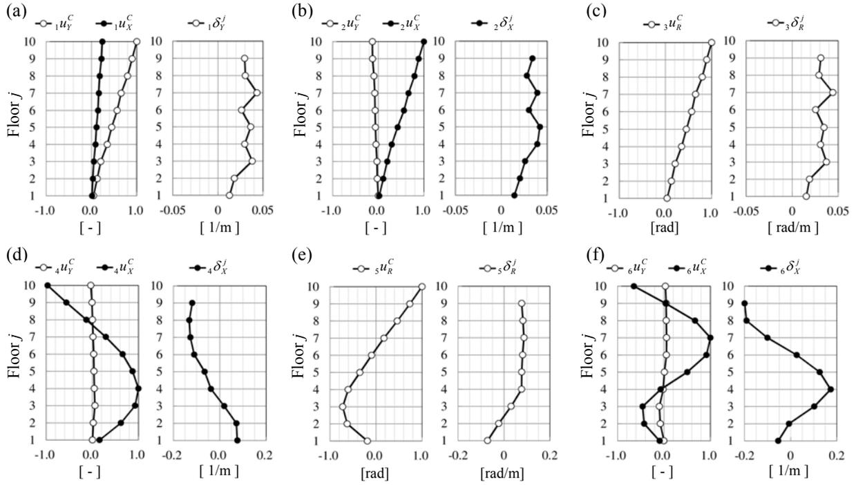
Figure 8. Mode shapes and modal deformation ratio at center of mass: (a) mode I, (b) mode II, (c) mode III, (d) mode IV, (e) mode V, and (f) mode VI
