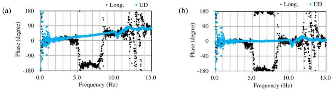
Figure 4. Phase of CSDF between two sensors: (a) before time correction and (b) after time correction
