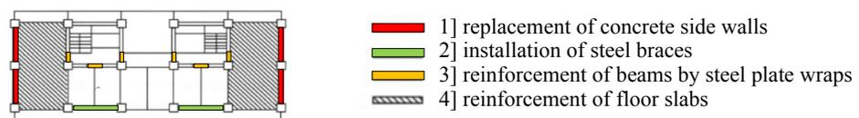
Figure 2. Seismic retrofitting from September 2000 over six months (Motosaka et al., 2002)
