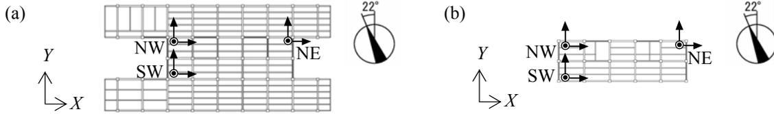
Figure 3. Location of accelerometers and indices: (a) first and second floors (lower floors), (b) floors above the second floor (upper floors)
