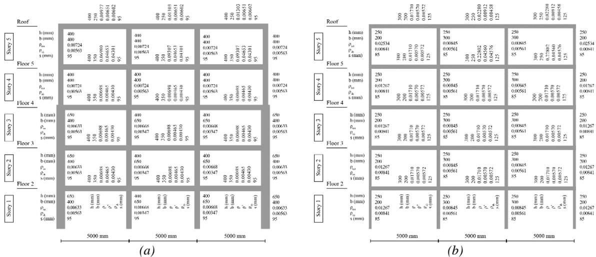
Figure 1. Geometric and steel detailing characterization of archetype building models, (a) Model No. 1 designed for special seismic considerations, (b) Model No. 2 designed for no seismic considerations
