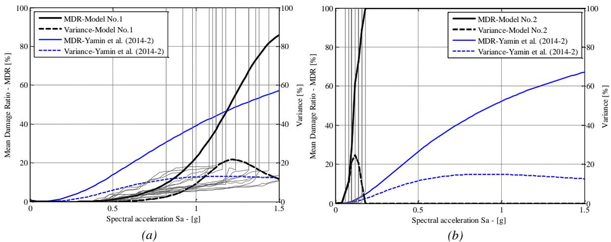
Figure 8. Vulnerability functions for the two archetype models, (a) Model No. 1 and (b) No. 2.
