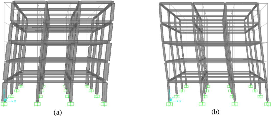
Figure 3. 3-D models for analysis and fundamental vibration modes (a) Model No. 1 and (b) Model No. 2
