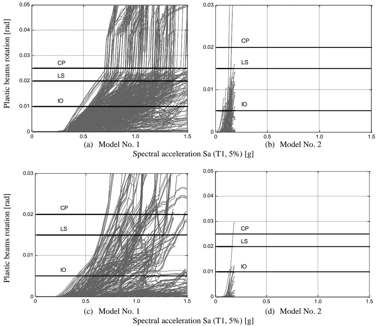
Figure 6. Plastic beam rotations for models (a) No.1, (b) No. 2 and plastic column rotations for models (c) No.1 and (d) No. 2
