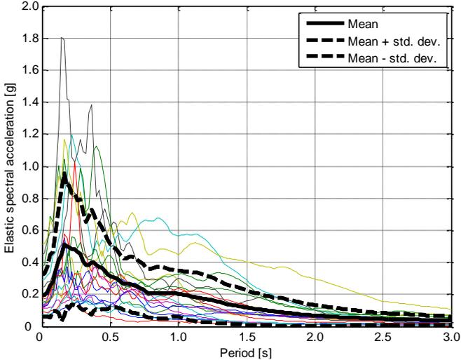
Figure 2. Elastic acceleration response spectrum for 5% damping of the selected records
