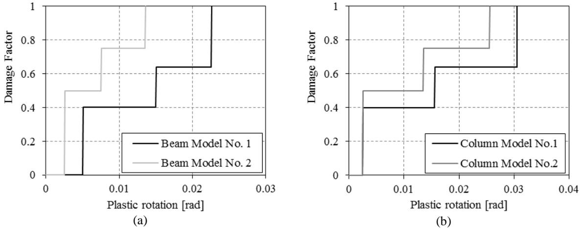
Figure 7. Representative damage functions for main structural elements a) Beams and b) Columns
