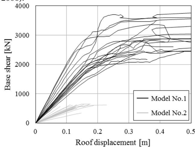
Figure 5. Incremental dynamic analysis (IDA) curves for Models No. 1 and No. 2
