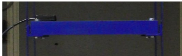
(b) Accelerometer attached to a floor
