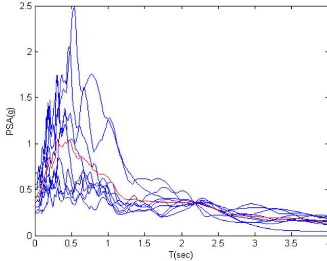
Figure 2. Pseudo Acceleration Spectra of the scaled records and the mean spectrum
