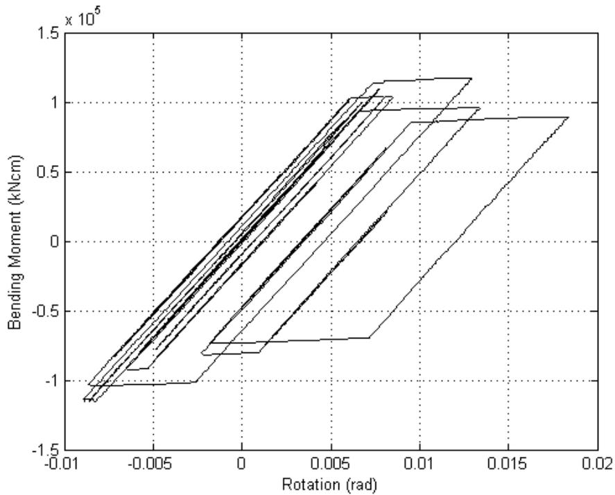
Figure 5. The first joint of the sixth floor's moment-rotation history for the degrading mode
