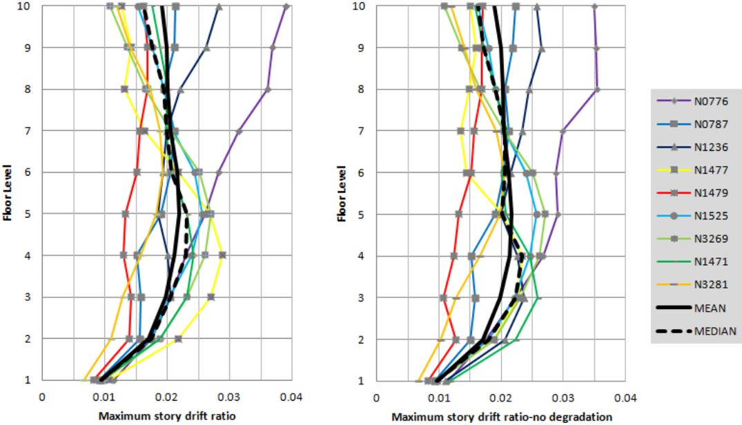
Figure 3. Story drifts, and mean and median values of story drifts obtained for the models with and without strength degradation
