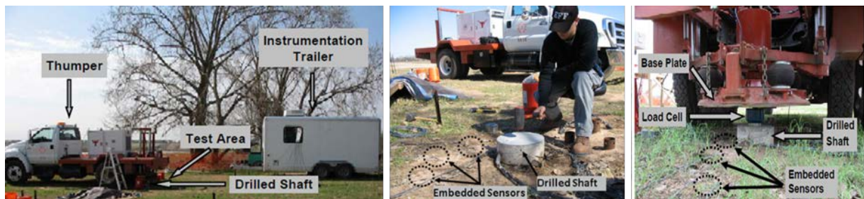
Figure 2. Dynamic testing using a variety of energy sources
