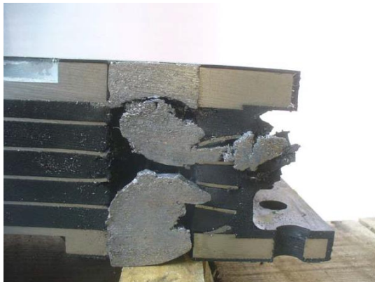
Figure 9. Fragmented lead plugs after DL2 test
