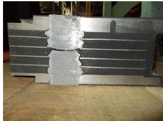
Figure 9. Fragmented lead plugs after DL2 test
