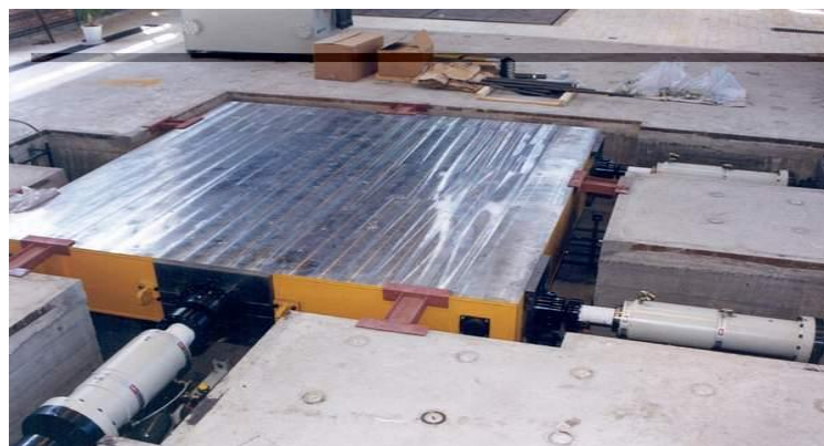
Figure 2. SST steel deck view consist of 3 hydraulic actuators
