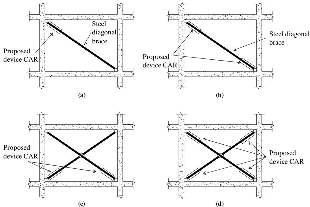
Figure 2. (a) One device CAR1 in single diagonal brace, (b) Two device CAR1 in single diagonal brace, (c) Two device CAR1 in cruciate diagonal steel rods, (d) Four device CAR1 in cruciate diagonal steel rods
