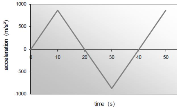
Figure 12. Diagram of load and time for time history analysis
