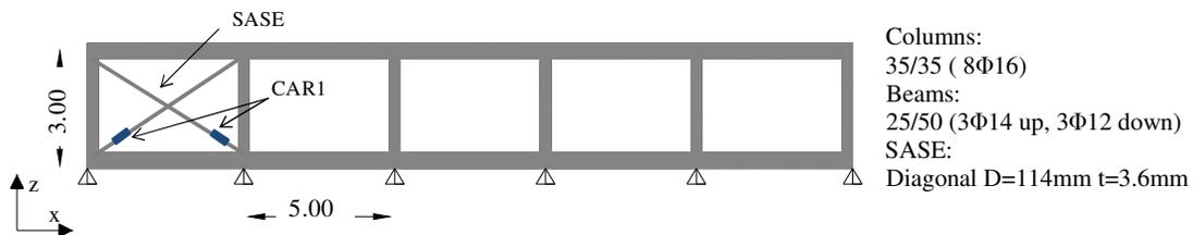
Figure 6. The one storey planar structural system DS1-CAR1
