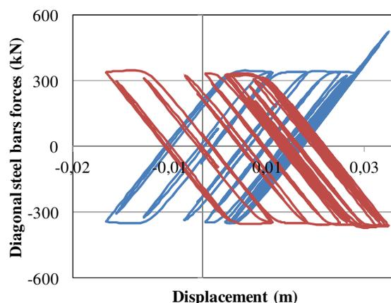
Figure 16. Axial forces of the diagonals steel rods of DS2-CAR1
