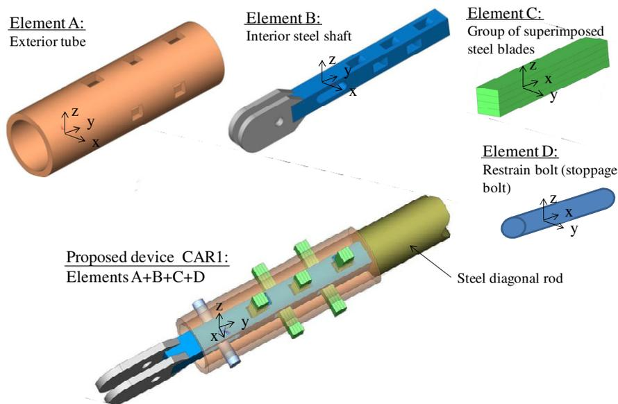
Figure 1. The parts of the CAR1 device
