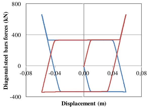
Figure 13. Axial forces of the diagonals steel rods of DS1-CAR1
