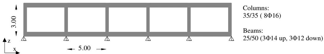
Figure 4. The one storey planar structural system BM1
