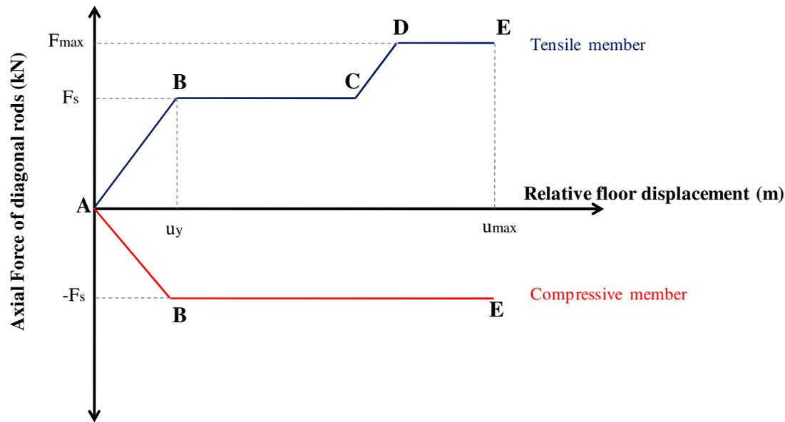
Figure 3. Non-linear multi-linear behaviour of the diagonal steel rods for tension and compression stress
