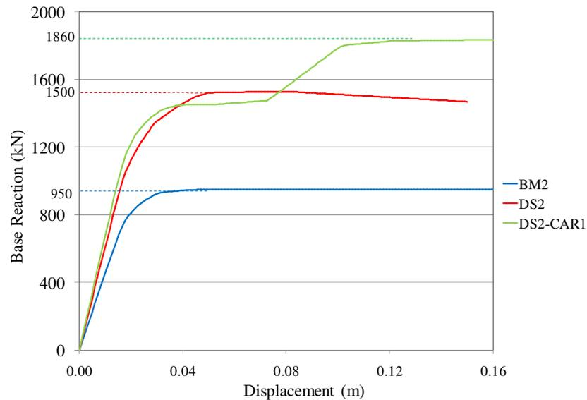
Figure 14. Push over curves of three storey planar structure
