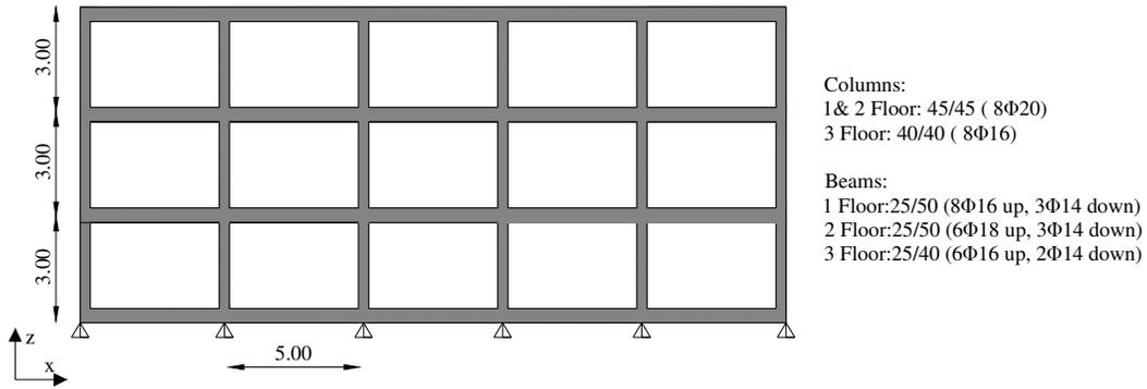
Figure 7. The three storey planar structural system BM2
