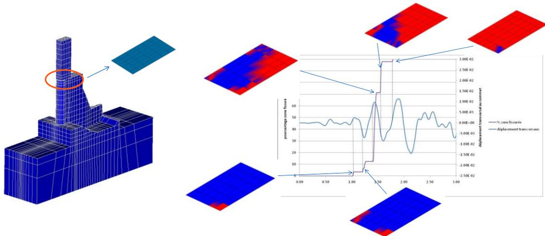
Figure 10 position of the joint-elements and spread of the crack during the ground motion
