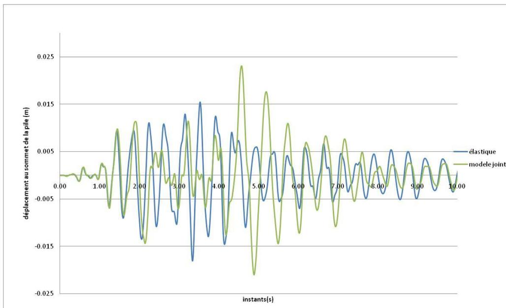
Figure 11 comparison of the side-to-side displacements on the top of the superstructure with the linear and non linear analysis
