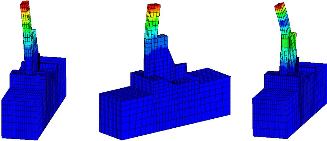
Figure 8 first eigenmode of the structure : 2.29 Hz, 6.43 Hz, 7.63 Hz
