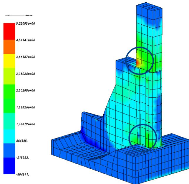
Figure 9 Maximum verticale tensile stresses during the earthquake
