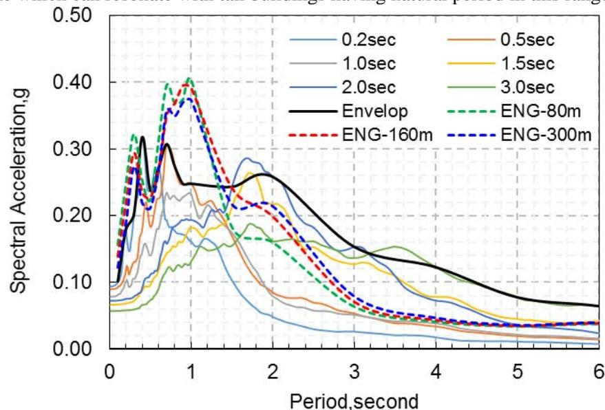
Figure 5. Average spectral response acceleration at surface for input ground motion matching with the conditional mean spectrum at 0.2, 0.5, 1.0, 1.5, 2.0 and 3.0 s
