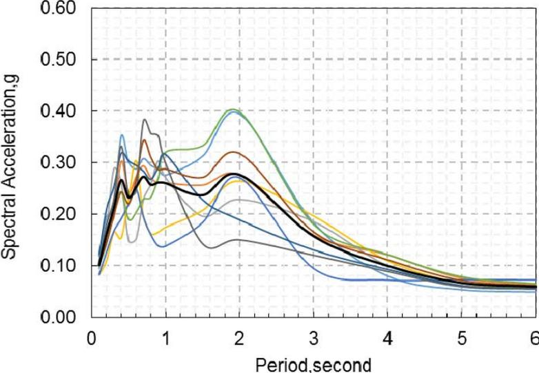
Figure 6.  $S_a$  of the observation sites (thin lines) and their average (thick line) in zone A
