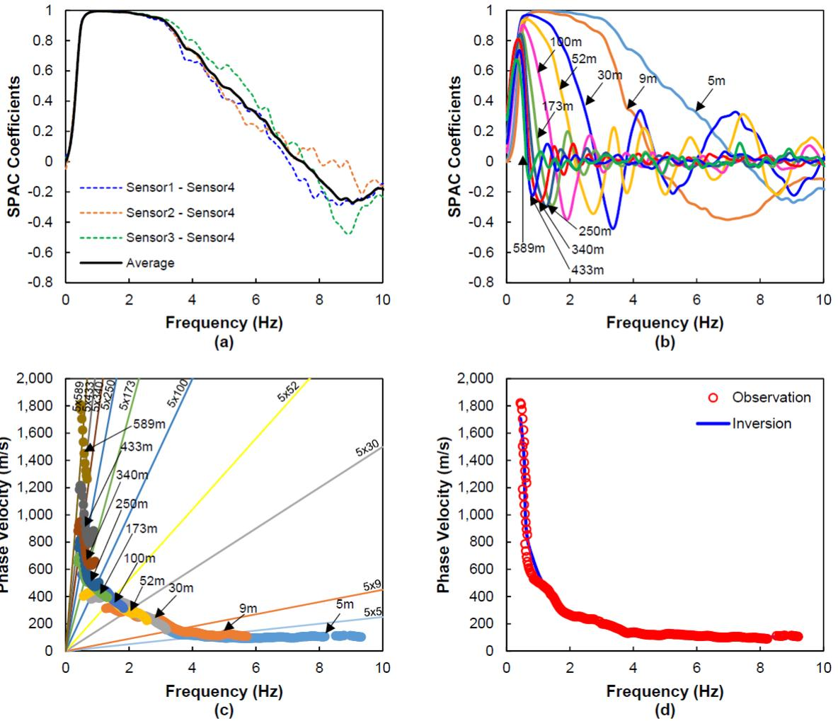
Figure 1. Example of SPAC analysis; (a) SPAC coefficients for 20-m array, (b) SPAC coefficients for all arrays, (c) dispersion curve for each array, and (d) final dispersion curve
