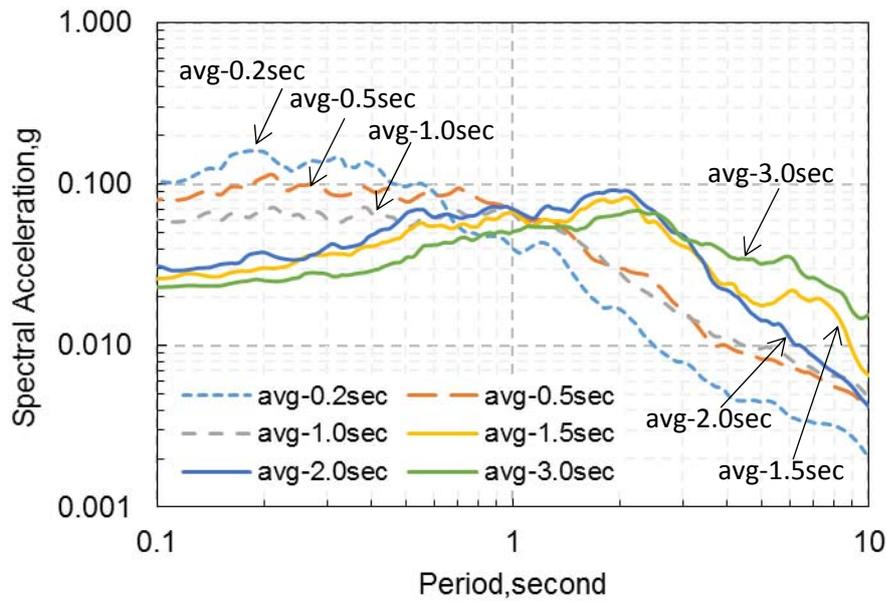
Figure 4. Average spectral response acceleration at rock outcrop of input ground motion matching with the conditional mean spectrum at 0.2, 0.5, 1.0, 1.5, 2.0 and 3.0 s
