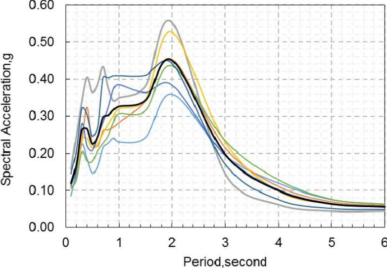
Figure 7.  $S_a$  of the observation sites (thin lines) and their average (thick line) in zone B
