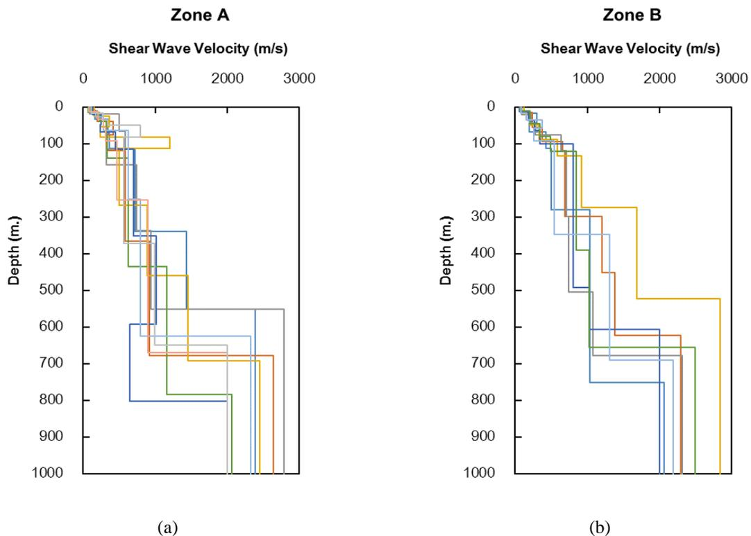
Figure 2. Shear wave velocity profile for 16 observation sites; (a) Zone A, and (b) Zone B
