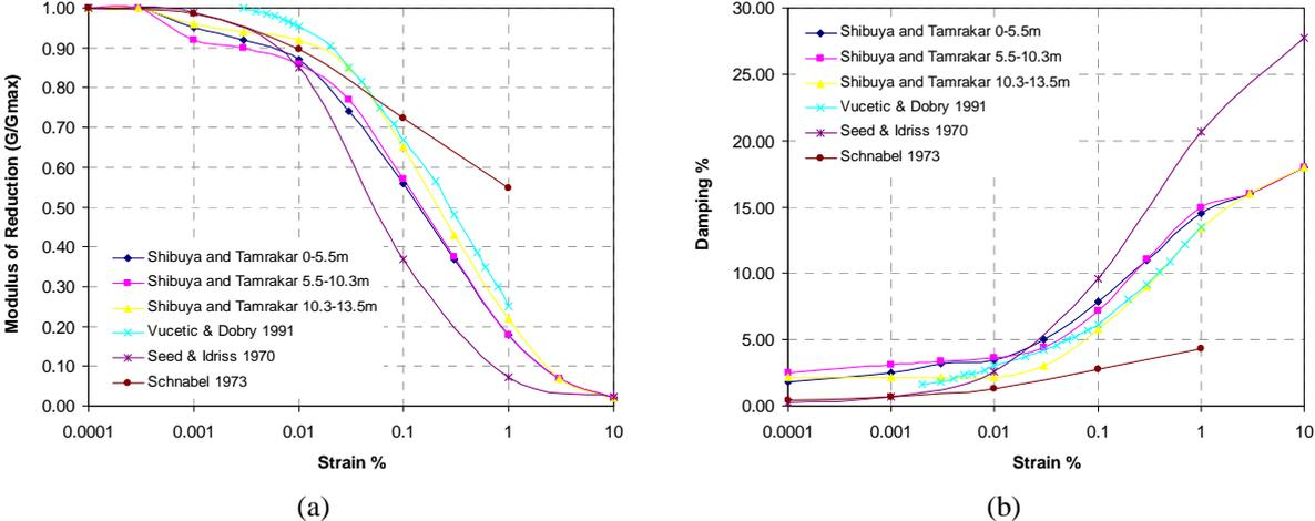
Figure 3. Dynamic properties of subsoil; (a) modulus reduction, and (b) damping
