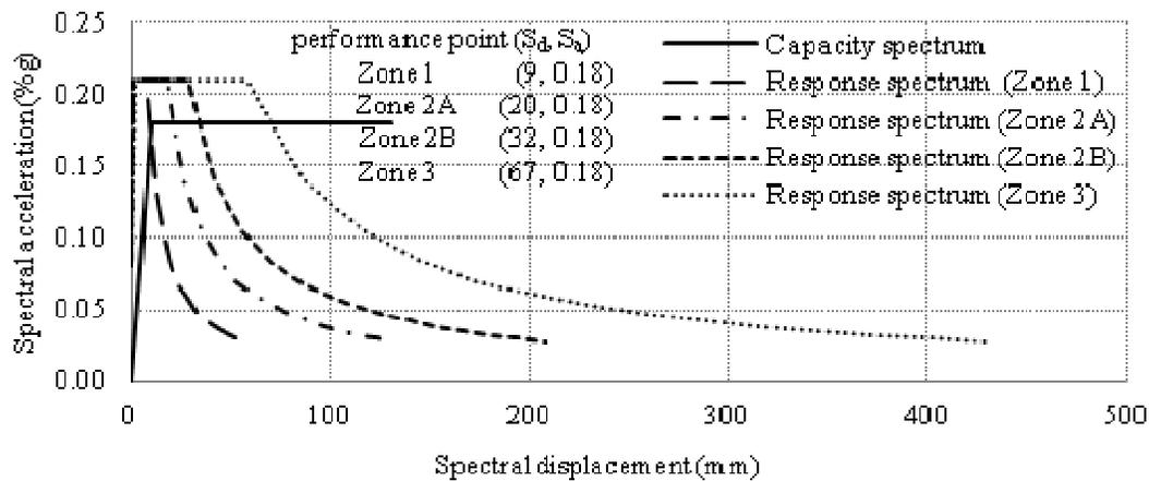
Figure 5. Constant ductility curves for the N-A3-L-R building
