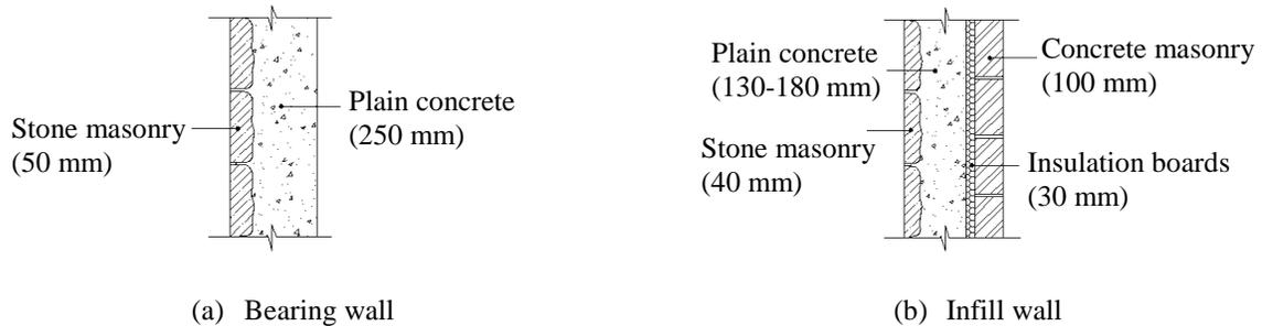
Figure 1. Cross-sectional details of stone-concrete walls
