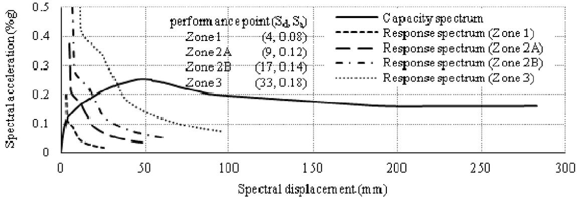
Figure 6. Application of the capacity spectrum method for the N-A3-L-R building
