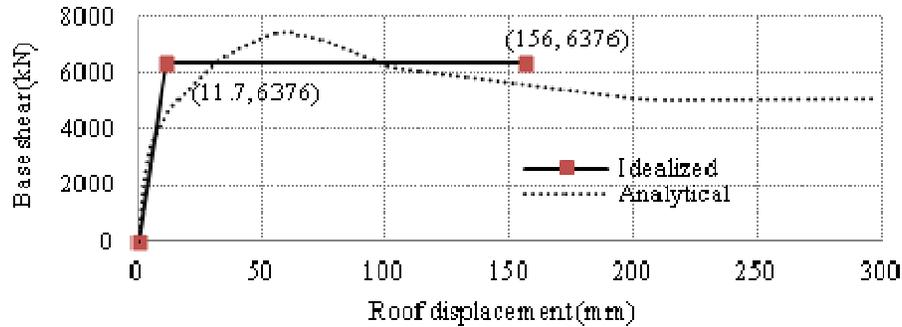
Figure 4. Bilinear idealization of the capacity curve of N-A3-L-R building
