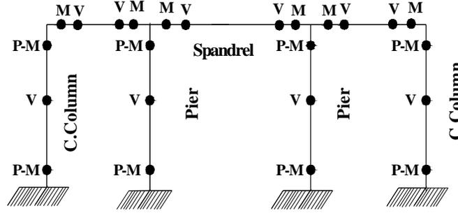
Figure 3. Locations of plastic hinges in piers, confining columns and spandrels
