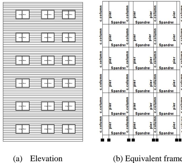
Figure 2. Equivalent frame modeling of a typical exterior bearing wall in building O-A1-M-R.
