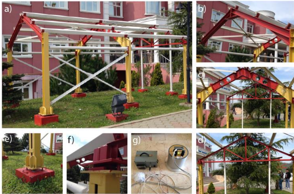
Figure 3. a) General layout b) Plate girder frame c) Castellated frame d) Truss frame e) Simple support f) Pin connection for truss frame g) Accelerometer GPS antenna and its power unit
