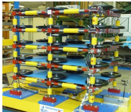
Figure 5. Frontal and lateral visualization of the shaking-table and the five floor 1:15 scaled structure.
