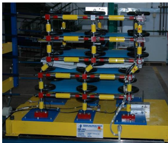
Figure 16 Mechanism pillars plasticized on the third floor of the model 5_M1 so as estimated by the method for damage localization.
