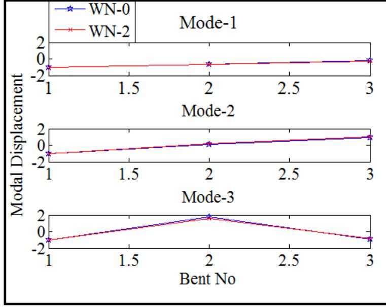
Figure 5: Identified Mode Shapes (WN-0 & WN-2)
