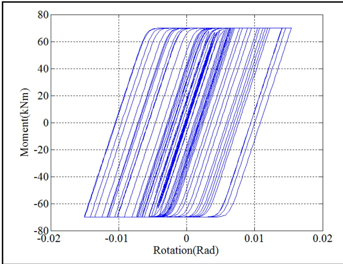
Figure 7: The Response of Bent-1 in Terms of Rotation
