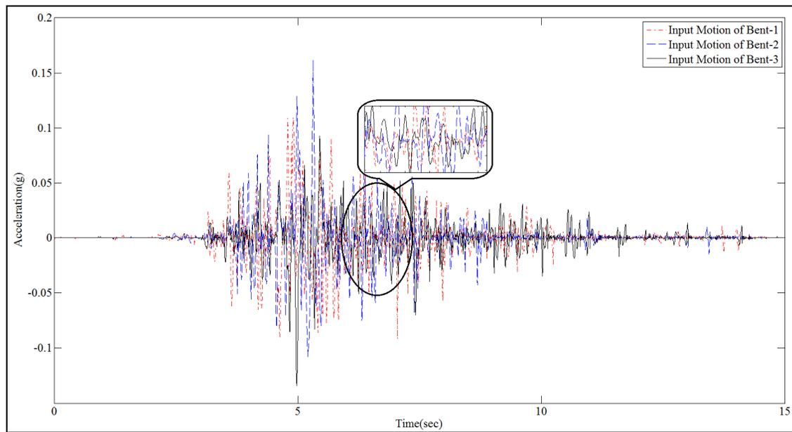
Figure 3: Different Input Motions of Test-1 for Three Bents
