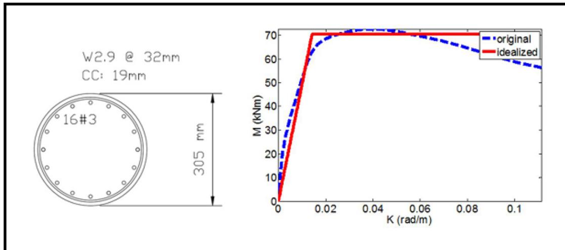
Figure 6: Cross-Sectional Properties and Moment-Curvature Relationship of Columns
