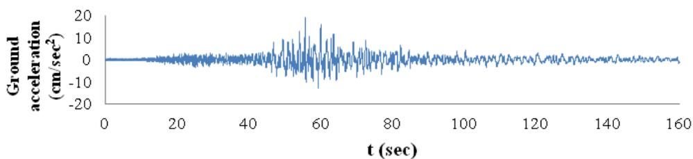
Figure 1. Ground motion time history used for dynamic non-linear analysis
