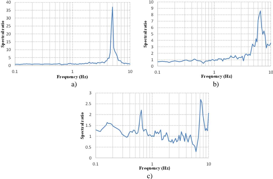
Figure 7. Spectral ratios estimated for the School building using ambient vibration; a) Longitudinal mode, b) Transversal mode, and c) Rotational mode
