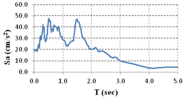
Figure 2. Pseudo-acceleration response spectrum with damping ratio equal to 0.05
