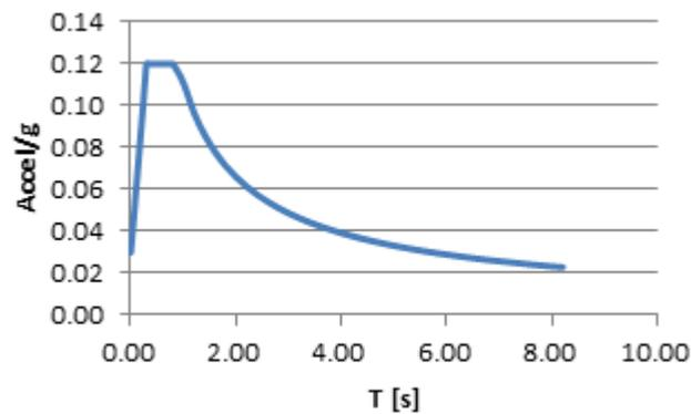
Figure 3. Acceleration design spectrum used for linear analysis
