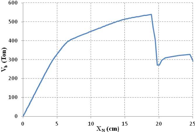
Figure 8. Pushover curve obtained from the School building (longitudinal direction)
