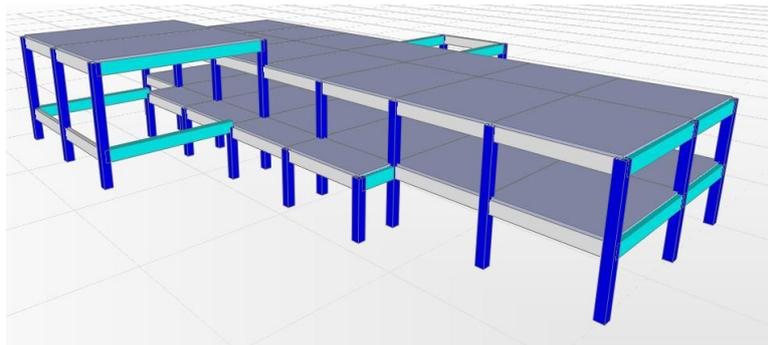
Figure 4. Structural model for the Hospital building developed in SAP2000 software
