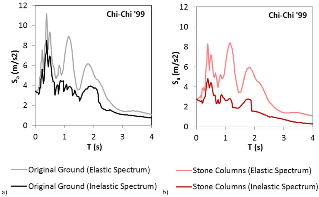
Figure 6 Elastic and inelastic response spectra (for the required ductility) based on the time-history at the middle of the foundation of the soil-foundation-structure models in the case of the original (a) and the improved (b) foundation ground.
