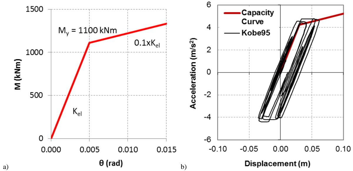
Figure 4. a) Backbone of the non-linear rotation spring at the superstructure. b) Loops of superstructure acceleration of the fixed-base yielding structure versus its relative displacement to its base.
