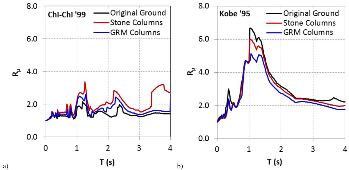
Figure 7 Force-reduction factor of the superstructure in the original and improved soil-foundation-structure system.
