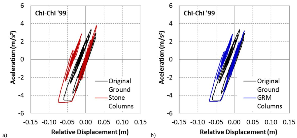
Figure 5. Loops of superstructure acceleration versus relative displacement to its foundation.
