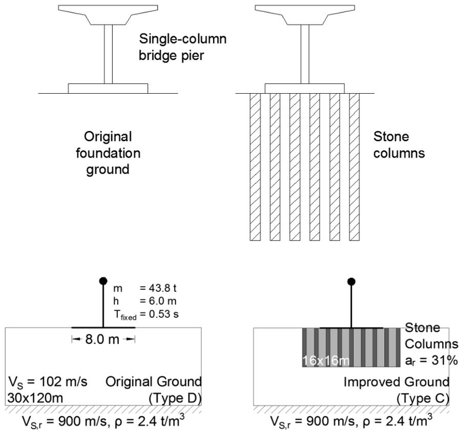
Figure 1. General schematics of the finite element models of the soil-foundation-structure systems
