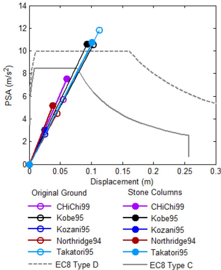
Figure 2. Performance points of the superstructure in the soil-foundation-superstructure models in the case of the original foundation ground and the improved with stone columns.
