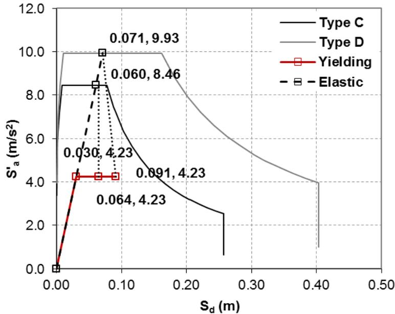
Figure 3. Performance assessment of the fixed-base structure based on Eurocode's spectra for the original (Type D) and the improved foundation ground (Type C).
