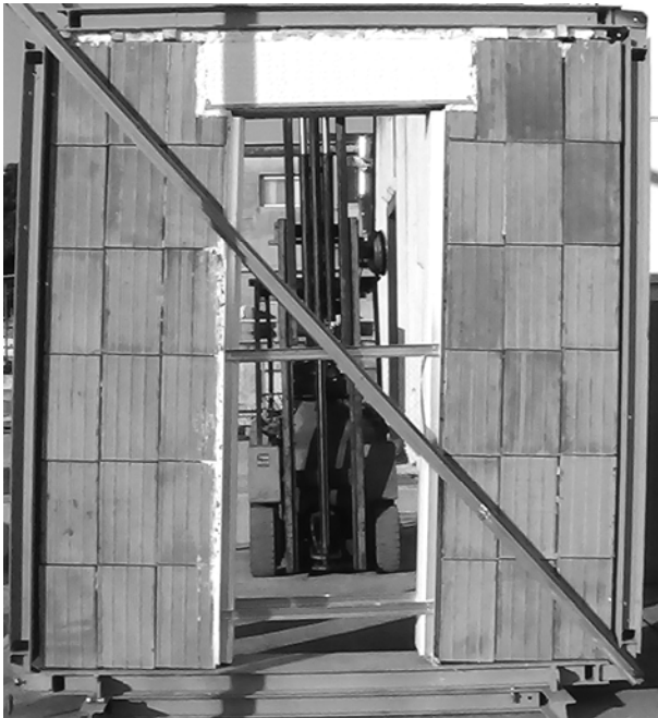
Figure 4. Cyclic behavior to collapse of joint assembled with bricks.
