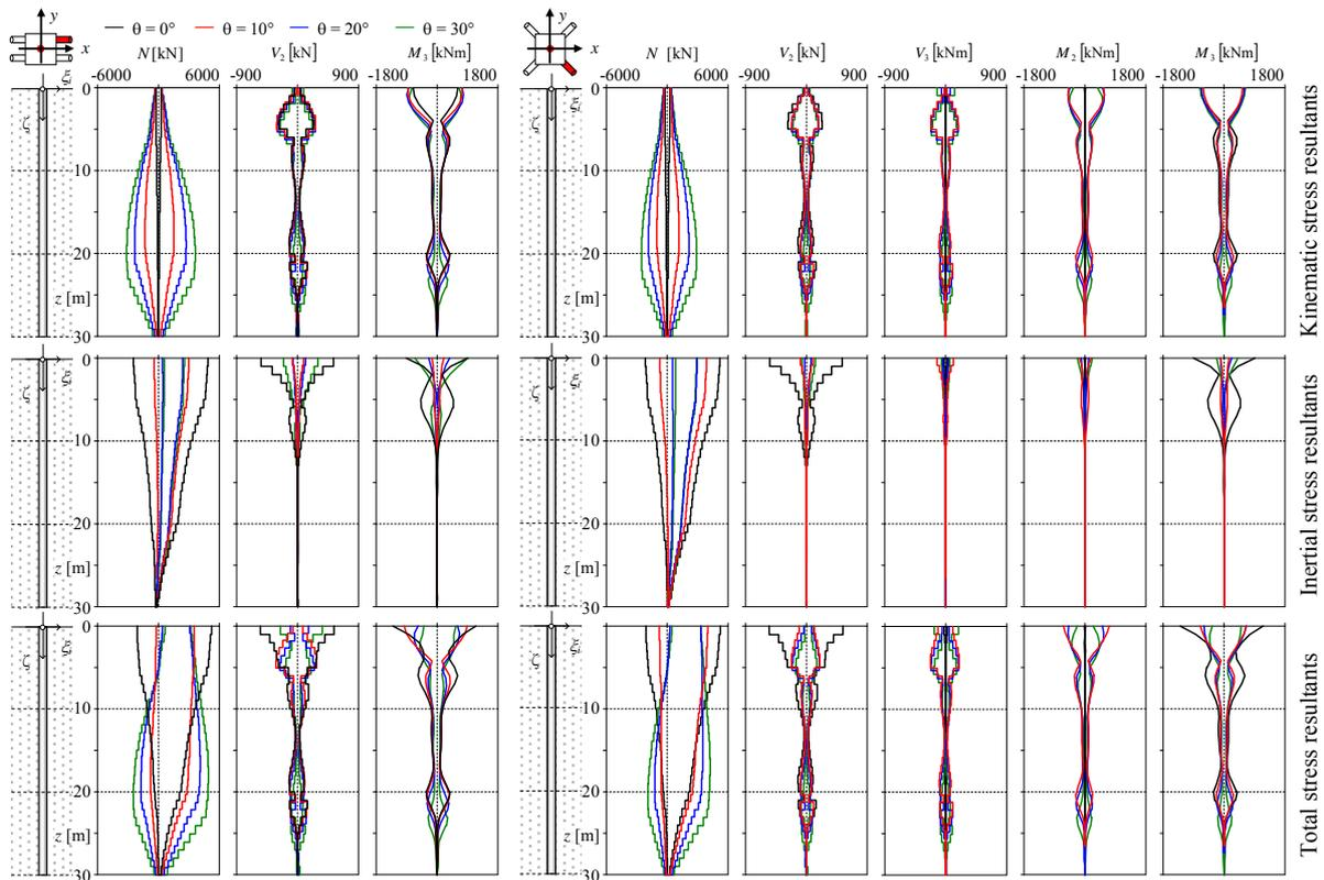
Figure 9. Pile stress resultants: kinematic, inertial and total components
