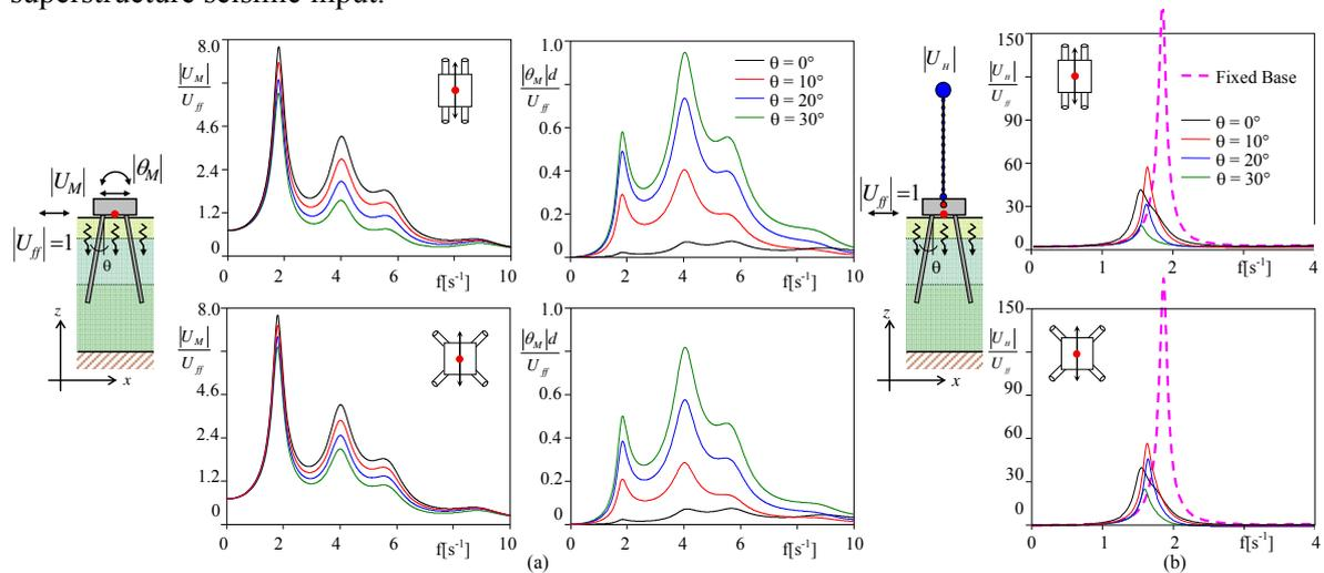
Figure 5. Frequency response: (a) displacement and rotation of the pile cap (“kinematic interaction”); (b) displacements of the pier head (“kinematic and inertial interaction”)
