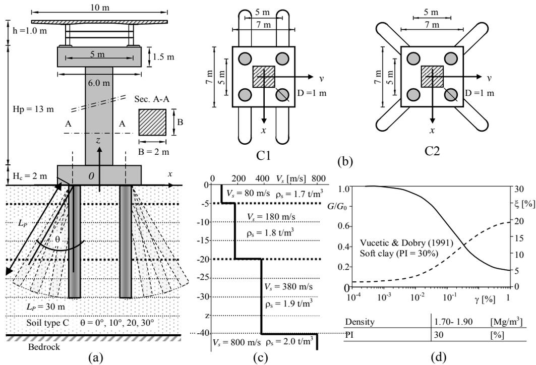
Figure 2. (a) Cross section of the soil-foundation-superstructure system; (b) foundations layouts; (c) shear wave velocity profile of the soil deposit and (d) shear modulus degrading and damping evolution curves
