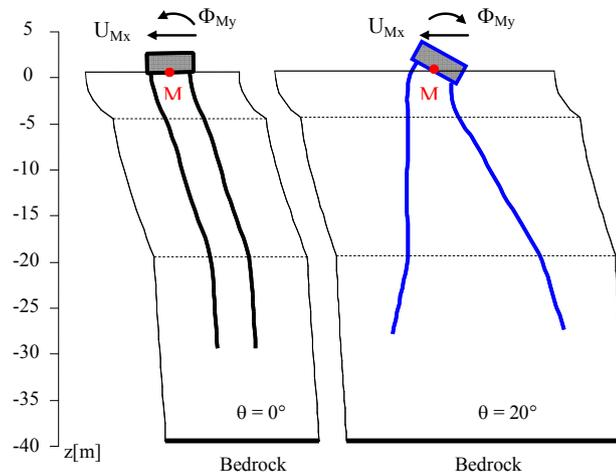
Figure 7. Deformed shape of the soil-foundation system (C1,  $\theta = 0^\circ$  e  $20^\circ$ ) subjected to the Campano-Lucano earthquake (Arienzo)
