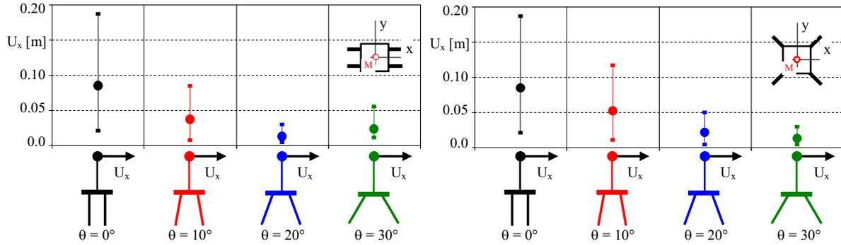
Figure 8. Mean absolute values of the superstructure displacements
