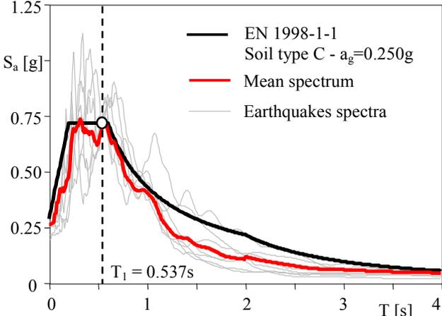
Figure 3. Acceleration elastic response spectra at the deposit surface: spectra of the selected earthquakes, mean and reference spectra
