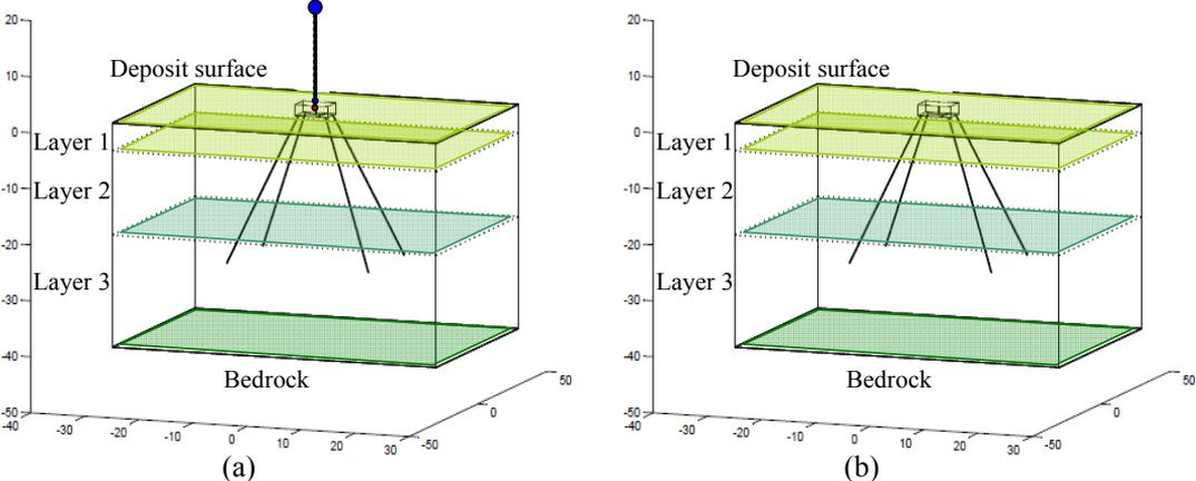
Figure 4. Developed numerical models: (a) soil-foundation superstructure model and (b) soil-foundation model for the evaluation of kinematic interaction effects
