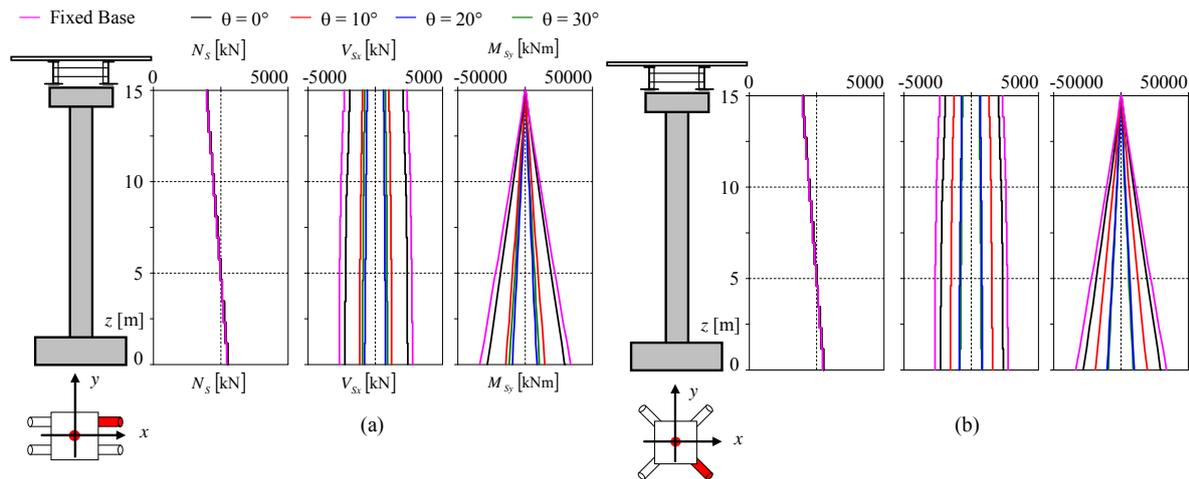
Figure 10. Superstructure stress resultants: (a) pile group configuration C1 and (b) C2
