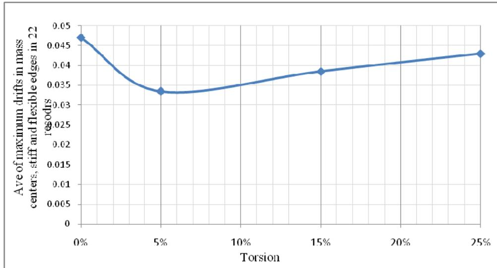
Figure. 8 The average of maximum story drift in mass centers, stiff and flexible edges with increase in the mass eccentricity
