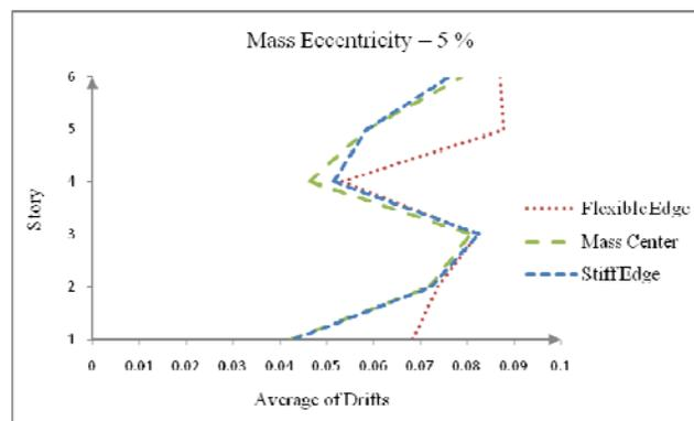
Figure 4. The average value of maximum story drifts in mass centers, stiff and flexible edges in an irregular building with mass eccentricity of 5% in presence of 22 earthquake records
