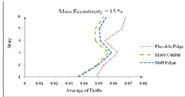
Figure 5. The average value of maximum story drifts in mass centers, stiff and flexible edges in an irregular building with mass eccentricity of 15% in presence of 22 earthquake records
