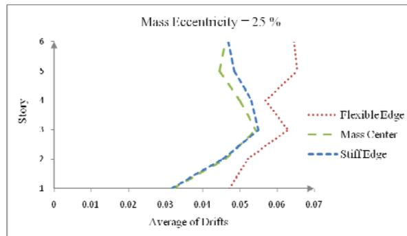
Figure 6. The average value of maximum story drifts in mass centers, stiff and flexible edges in an irregular building with mass eccentricity of 25% in presence of 22 earthquake records
