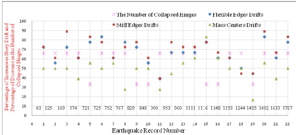
Figure. 9 The percentage of the number of collapsed hinges and story drifts increase in the mass centers, stiff and flexible edges with increase in the mass eccentricity in plan
