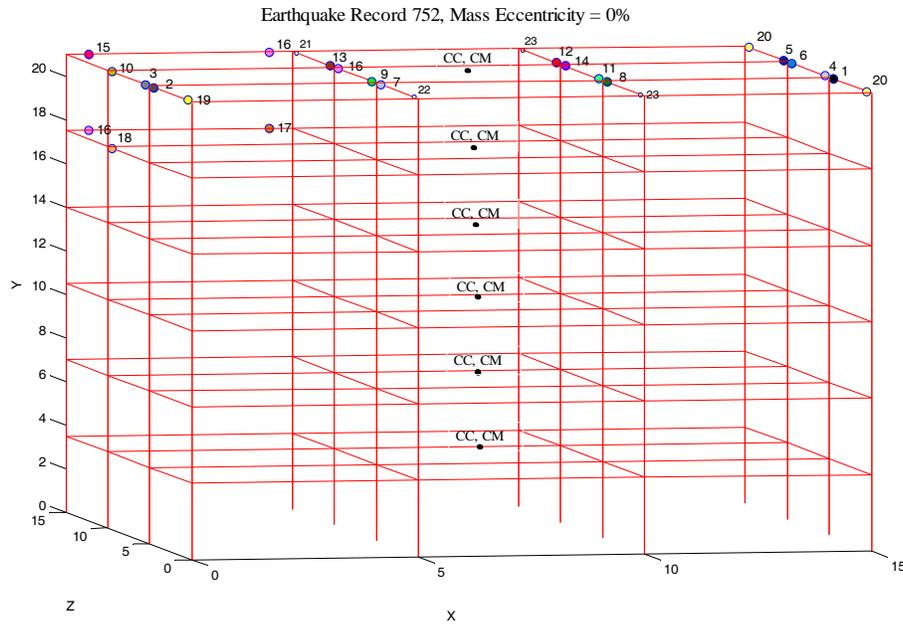
Figure 1. Collapse distribution in a regular building in presence of the ground motion record #752
