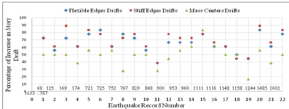
Figure. 7 The percentage of increase in story drift in mass centers, stiff and flexible edges with increase in the mass eccentricity
