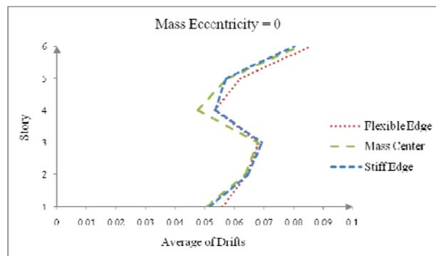
Figure 3. The average value of maximum story drifts in mass centers, stiff and flexible edges in a regular building in presence of 22 earthquake records
