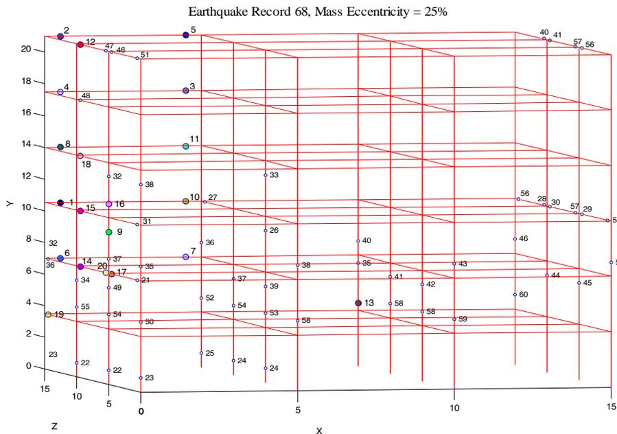
Figure 2. Collapse distribution in an irregular building with mass asymmetry of 25% in presence of the ground motion record #68
