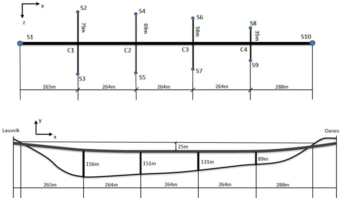
Figure 2. Plan and elevation of the Høgsfjord tunnel; S1-S10 represent the supports.
