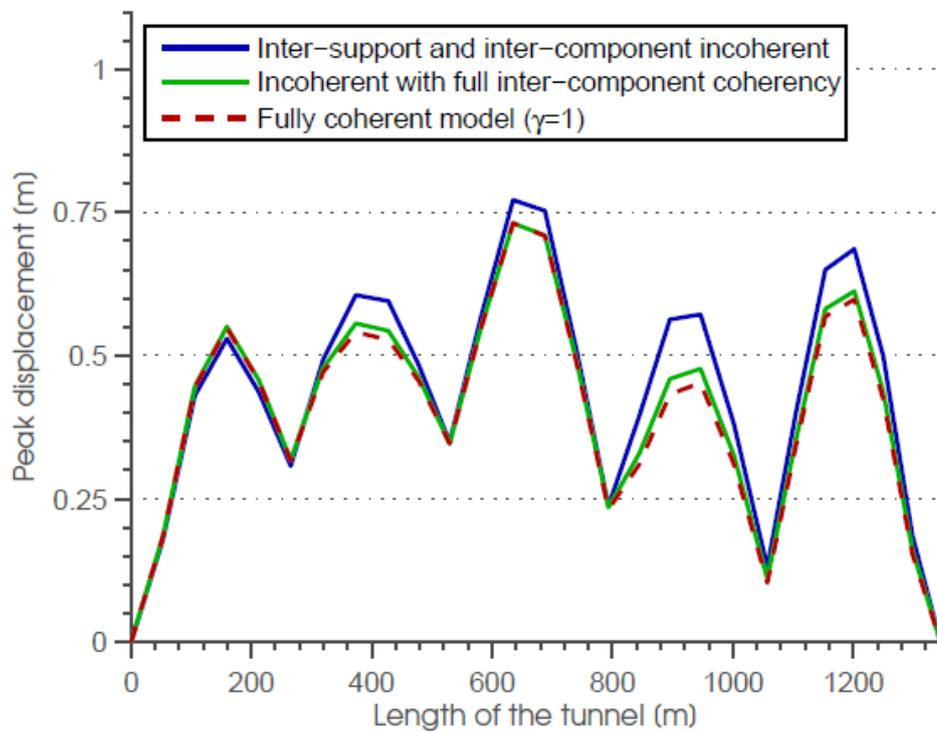
Figure 4. Expected peak vertical displacement along the length of the tunnel; seismic waves are propagating parallel to the tunnel axis a velocity of 500m/s.
