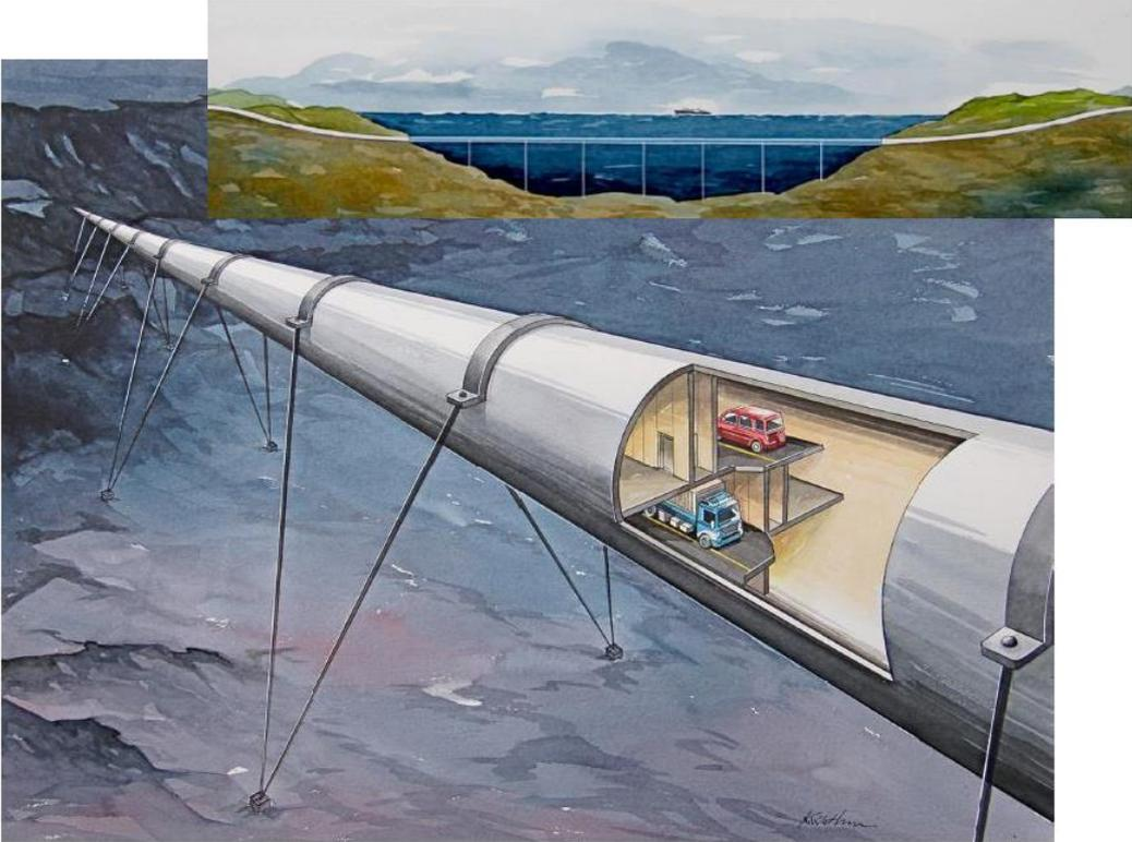
Figure 1. Artist’s sketch of an anchored submerged floating tunnel (NPRA, 2011; NRPA, 2012)
