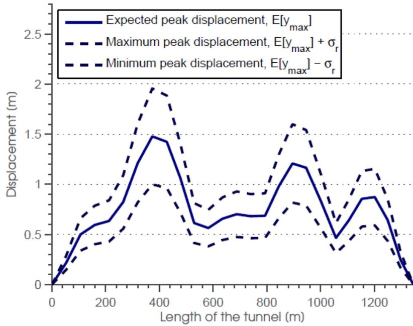
Figure 3. Peak transverse displacement along the length of the tunnel; seismic waves are propagating parallel to the tunnel axis a velocity of 500m/s. The solid trace represents the expected value while the two dashed ones correspond to the expected value plus (minus) one standard deviation.
