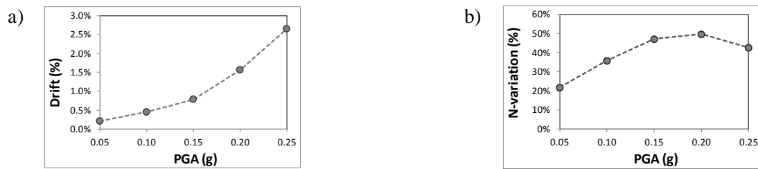
Figure 2. Drift at the 1 st storey and axial load variation (pushover analysis).
