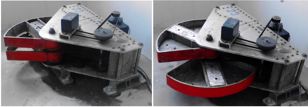
Figure 2. GSV-101 (Geotronix, USA) – position of the shaker baskets for maximal excitation force (left) and zero excitation force (right)
