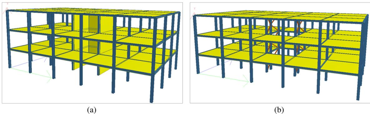
Figure 2. Axonometric view of (a) Swedish model with reinforced concrete core; (b) Swedish model with steel bracing
