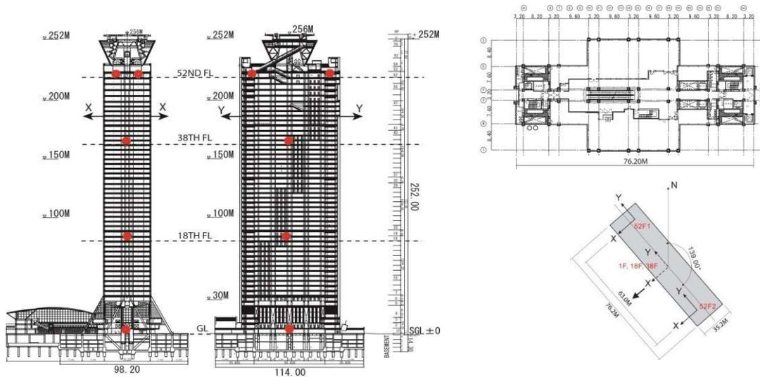
Figure 3. (Left) Vertical sections and plan views of the building showing major dimensions and locations of tri-axial accelerometers on the 52n, 38th, 18th and ground level (1st Floor). X and Y denote principal axes of the building (from [8]). (Right Top) Typical plan view (the figure shows 52<sup>nd</sup> floor) and (Right Bottom) orientations (from [8]).
