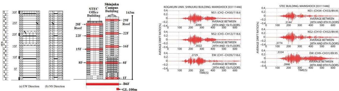
Figure 8. (left) Vertical sections showing instrumented floors of Building C (30 story Shinjuku Campus Building) and Building D (28 story STEC Office Building) in Shinjuku area of Tokyo, Japan (Figure adopted from [Hisada et al, 2012a and b]). (Center and Right) Average drift ratios computed from recorded data of Building C and D.
