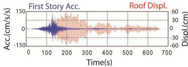
Figure 7. Recorded first story accelerations (max ~14% of g) and computed roof displacements (max ~ 54cm) during Tohoku earthquake (figure adopted from J. Moehle and Y. Sinozaki).
