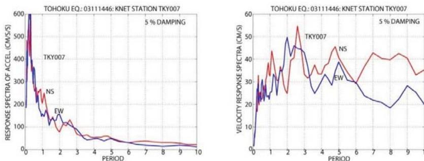
Figure 2. (left) NS and EW acceleration response spectra and (right) velocity response spectra of ground motions recorded during Tohoku event at KNET TKY007 station (Shinjuku, Tokyo) where tall buildings are concentrated. Velocity response spectra exhibit large amplitudes particularly for periods > 2 seconds.
