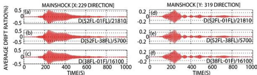
Figure 5. Average drift ratios computed from displacements between 52nd, 38th and 1st floors. In each frame, the numbers in denominators are distances (in cm) between the designated floors.
