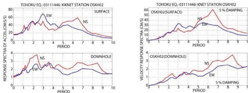
Figure 1. (left) NS and EW acceleration response spectra and (right) velocity response spectra of ground motions recorded at surface and downhole during Tohoku event at KIKNET OSKH02 station in Osaka Bay. Velocity response spectra exhibit the large amplitudes between 5-7 seconds.
