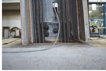
Figure 8. Gap opening of specimen WF1 at 5.0% rad drift
