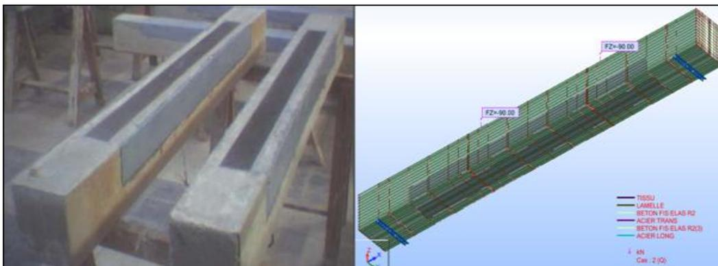
Figure 6. The second combination of strengthening (SB2 experimental and FE model)
