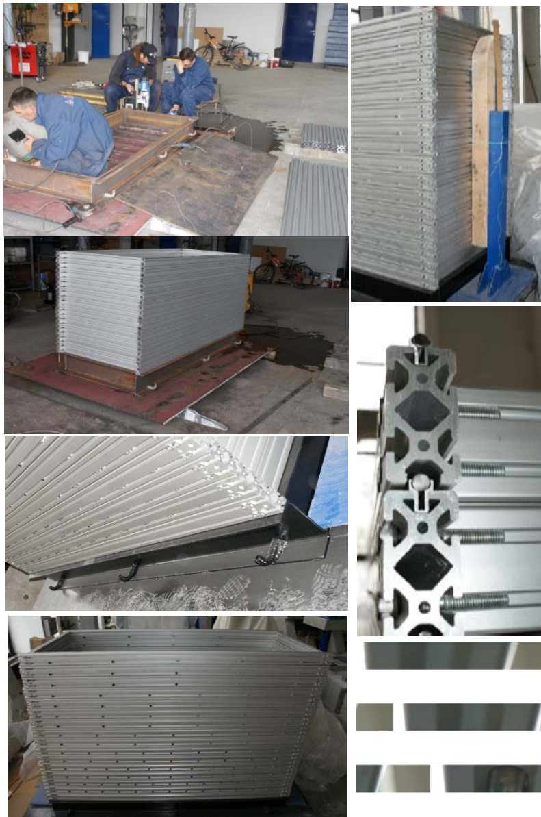
Figure 2 The construction process of the laminar box
