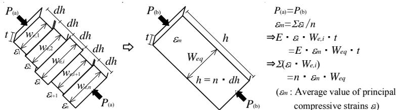
Figure 11. Equivalent diagonal strut width
