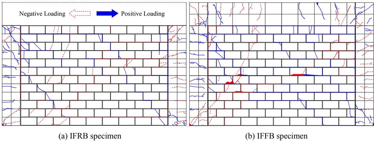
Figure 6. Crack patterns in both specimens
