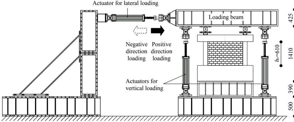
Figure 4. Test setup of IFFB specimen (Unit: mm)
