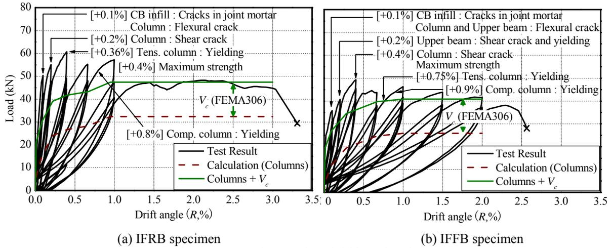
Figure 5. Lateral strength and drift angle relation
