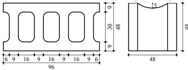
Figure 3. Details of small scale CB unit (unit: mm)
