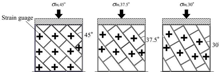
Figure 15. Element experiments with CB prisms
