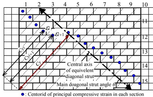
Figure 13. Central axis of diagonal strut
