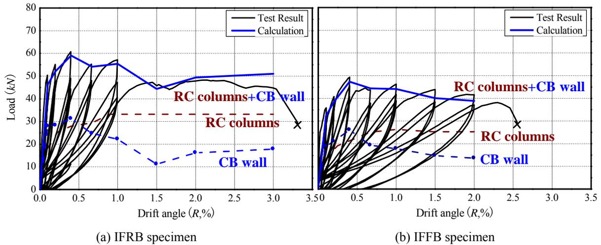
Figure 17. Lateral strength evaluation of both specimens
