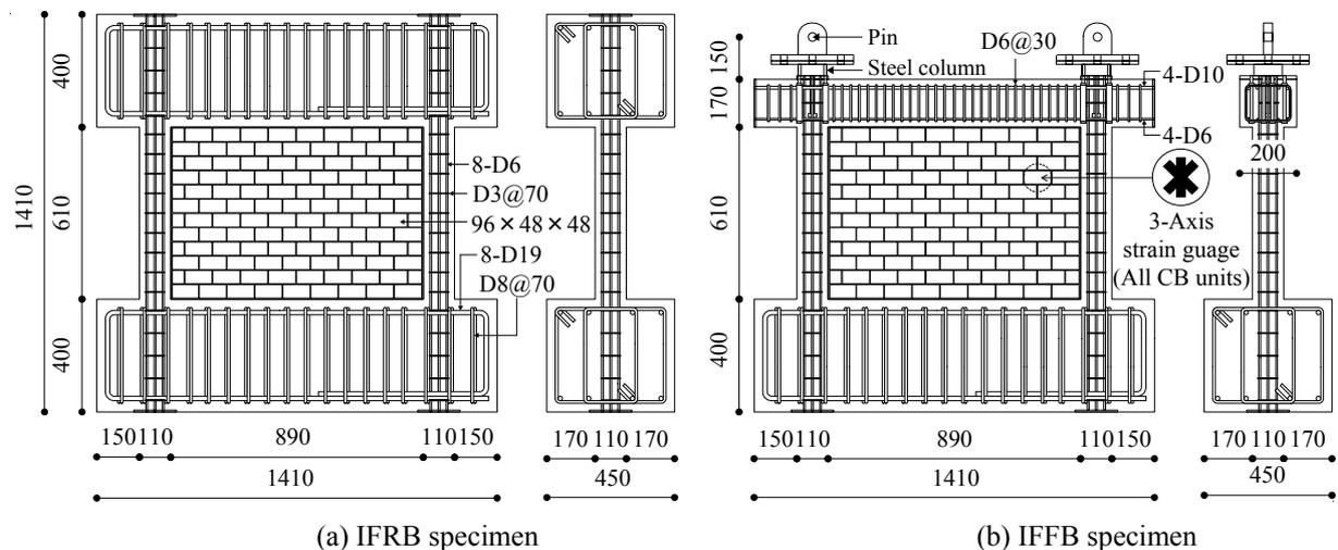
Figure 2. Details of specimens (unit: mm)
