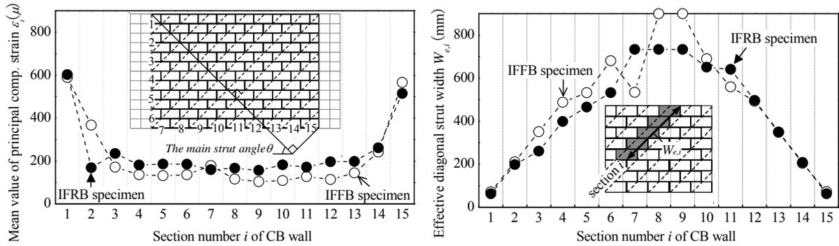
Figure 9. Mean value of comp. strain in each section (0.4%) Figure 10. Effective strut width in each section (0.4%)
