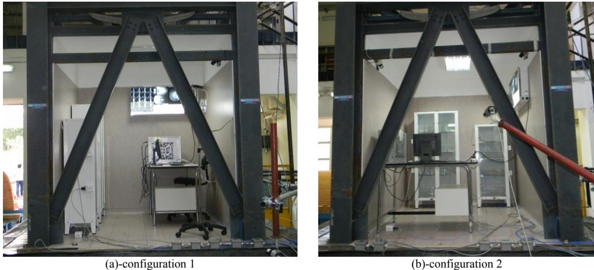
Figure 4. Photo of the test setup: (a) configuration 1, adopted in test groups 1000, 2000 and 3000 and (b) configuration 2, adopted in test groups 4000, 5000 and 6000.
