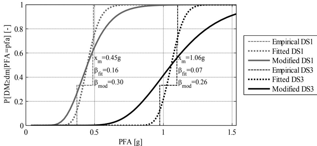
Figure 6. Fragility curves for the damage states 1 and 3 considering mass variability.
