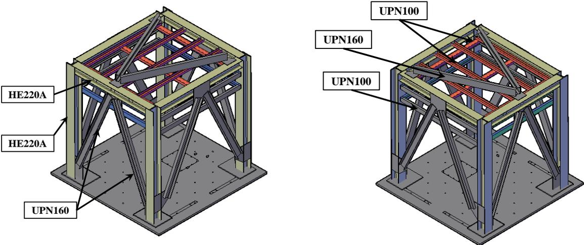
Figure 1. Global perspective of the test setup.
