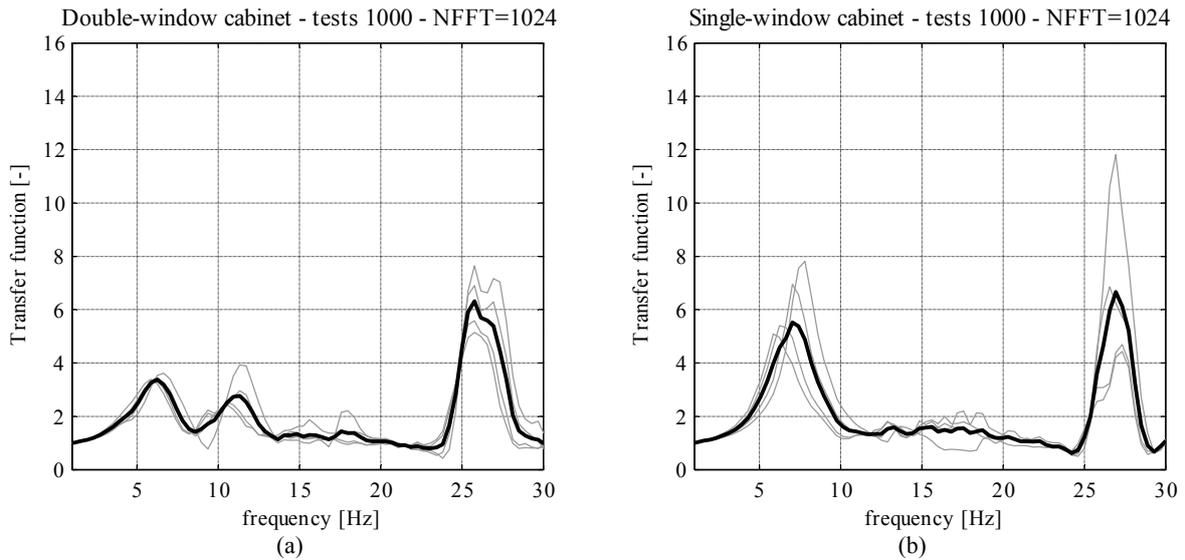
Figure 5. Transfer curves for (a) double-window cabinet – tests 1000, (b) single-window cabinet – tests 1000.
