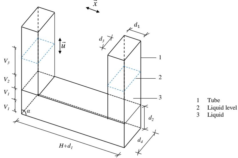
Figure 3. Drawing of a horizontally excited passive tuned liquid column damper with different horizontal and vertical cross-sections
