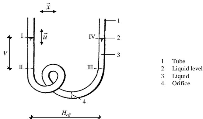
Figure 2. Drawing of a horizontally excited tuned liquid column damper from the patent document of Sakai
