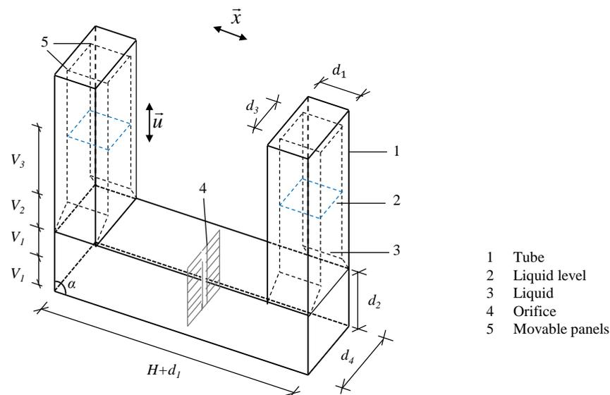
Figure 4. Drawing of a horizontally excited semiactive tuned liquid column damper with movable panels to tune its frequency
