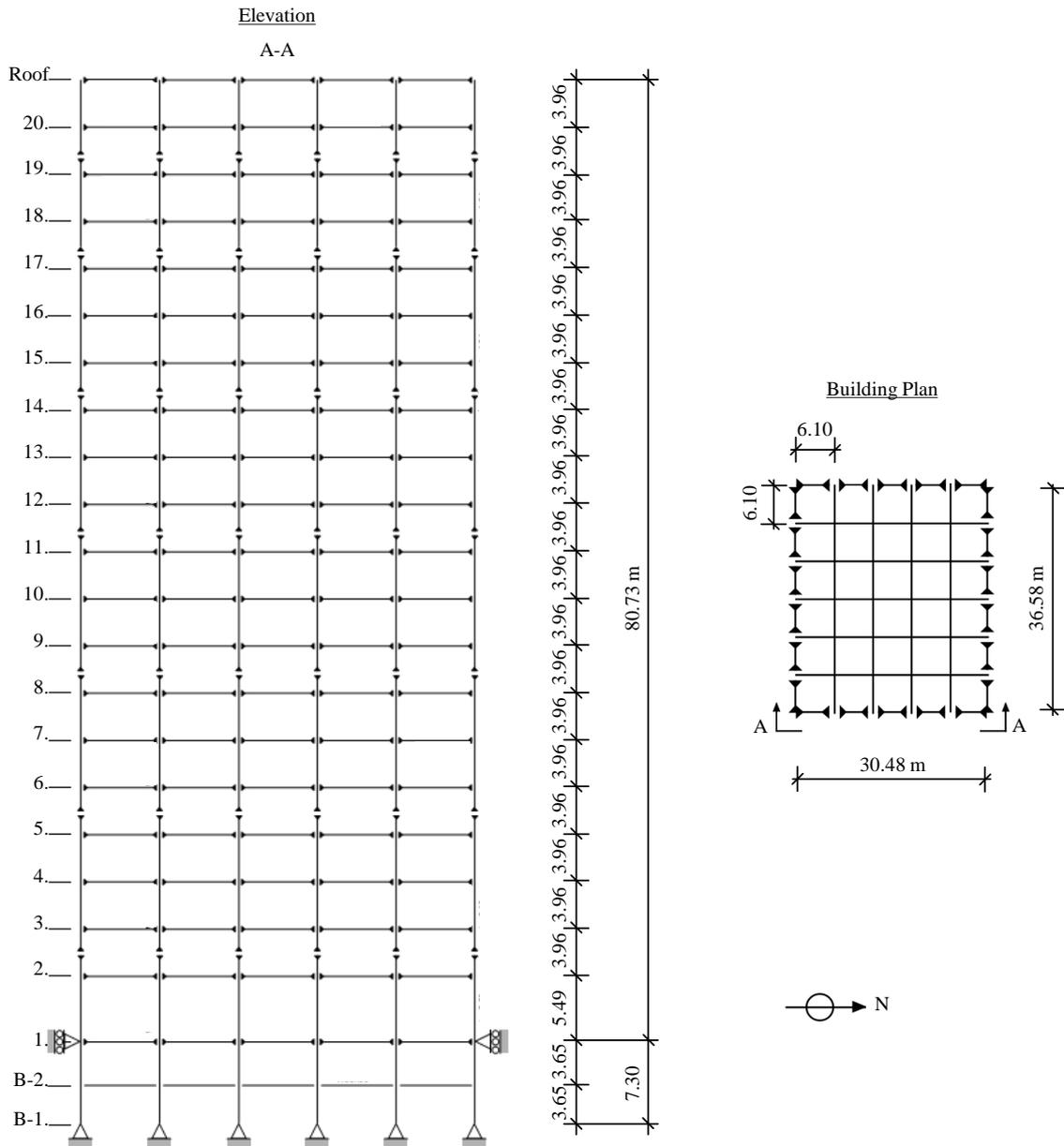
Figure 5. The 20-story steel frame benchmark building (Spencer et al., 1998)
