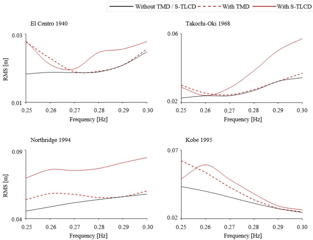
Figure 9. RMS values of the seismic roof deflection of the benchmark building without structural control, with S-TLCD and with an equivalent passive TMD-system
