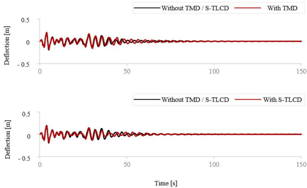
Figure 7. Time history of roof deflection of the benchmark building without structural control, with S-TLCD and with an equivalent passive TMD-system – El Centro earthquake, fundamental building frequency 0.26 Hz
