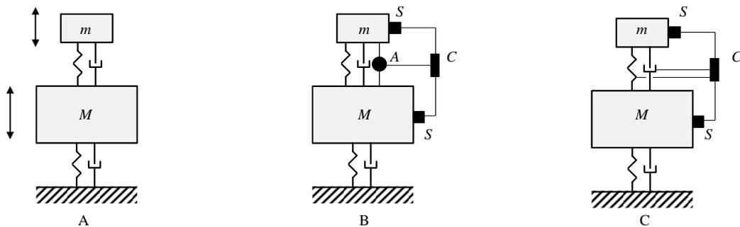
Figure 1. Passive (A), active (B) and semiactive (C) tuned mass damper attached to a primary structure
