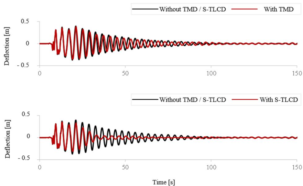
Figure 8. Time history of roof deflection of the benchmark building without structural control, with S-TLCD and with an equivalent passive TMD-system – Kobe earthquake, fundamental building frequency 0.26 Hz
