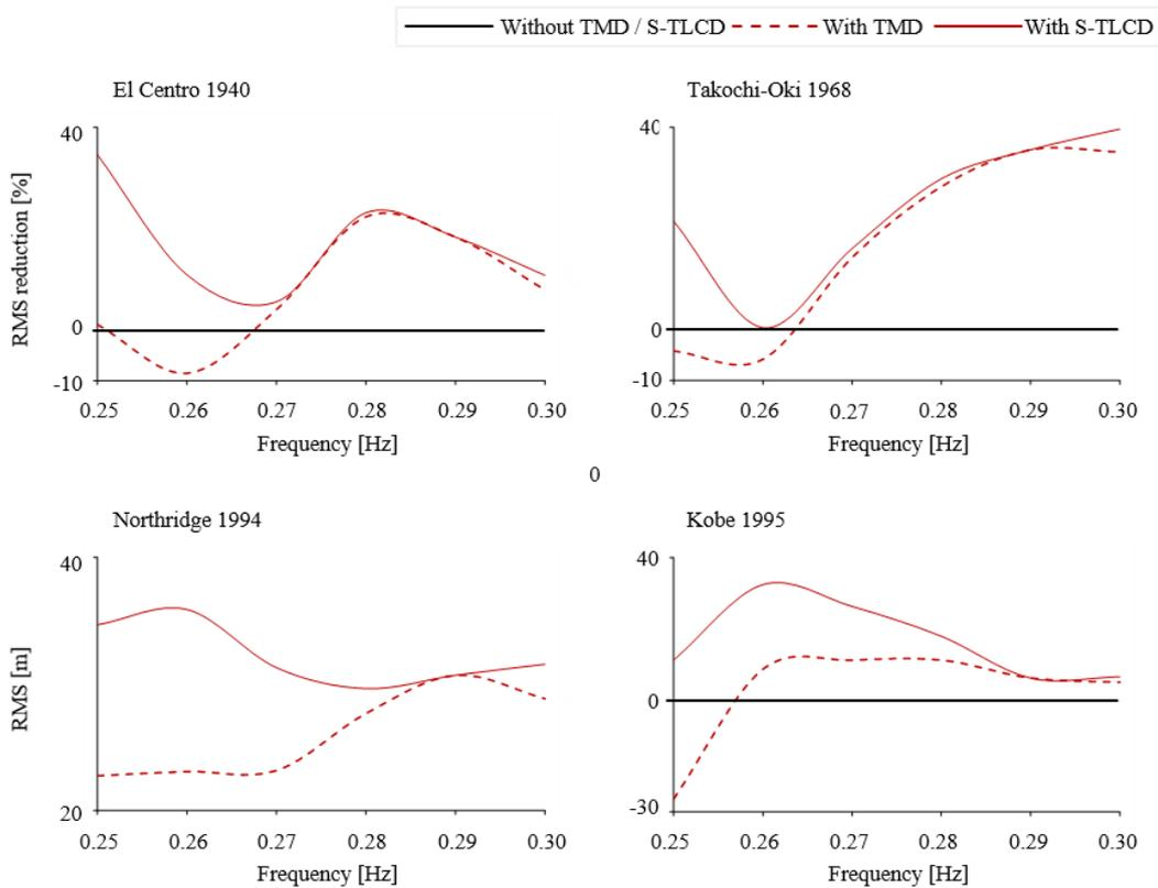
Figure 10. Reduction of the RMS values of the seismic roof deflection of the benchmark building without structural control, with S-TLCD and with an equivalent passive TMD-system
