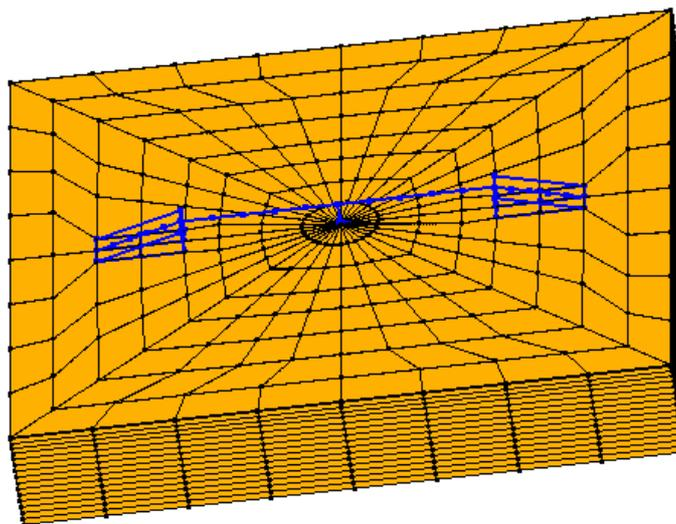
Figure 3 – Soil-Structure FEM model
