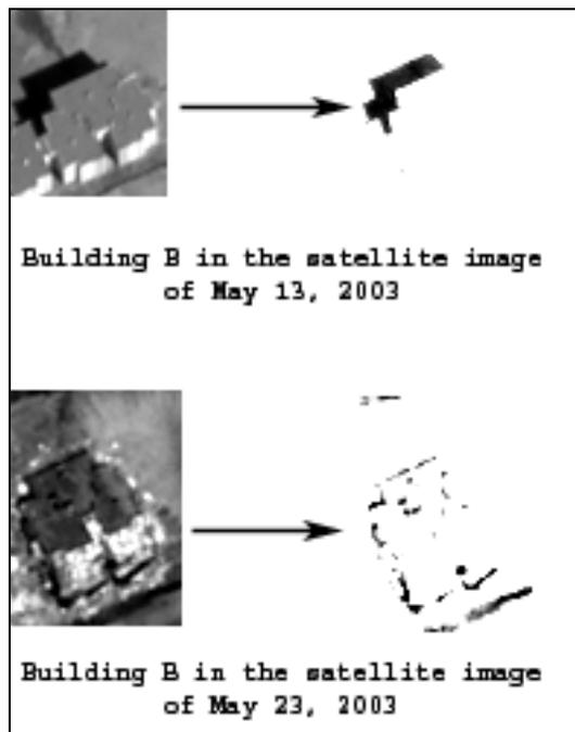
Figure 7. Extraction of building shadow in B
