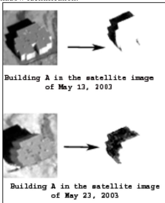
Figure 6.Extraction of building shadow in A
