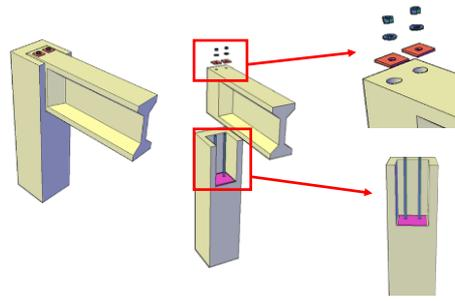
Figure 1. Beam-to-column dowel connection
