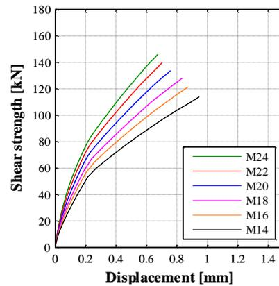
Figure 23. Shear force against the concrete cover: force-displacement curves varying the dowels diameter
