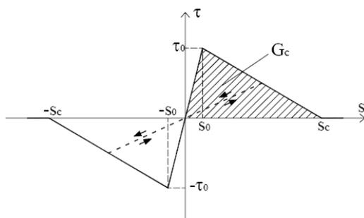
Figure 15. Adopted analytical model for cohesive interface elements
