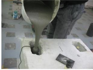
Figure 3. Cast of grout in the beam holes
