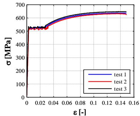
Figure 14. Experimental stress-strain relationships for steel reinforcement ( $\phi=8\text{mm}$ )
