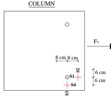
Figure 19. Layout of the strain gauges on the column top surface
