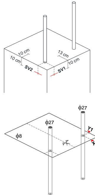
Figure 10. Geometrical layout of the column instrumentations
