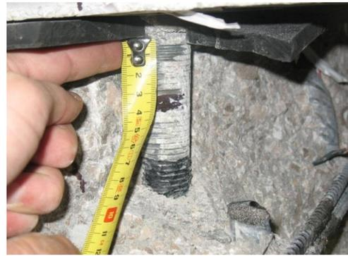
Figure 21. Measurement of the plastic hinge depth in the steel dowel after the monotonic test
