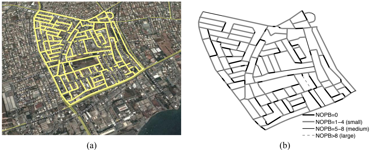
Figure 4 (a) aerial view of the DMA studied, (b) Graph model of a DMA of the water network of Limassol, Cyprus. The plot shows also the NOPB of every pipe.
