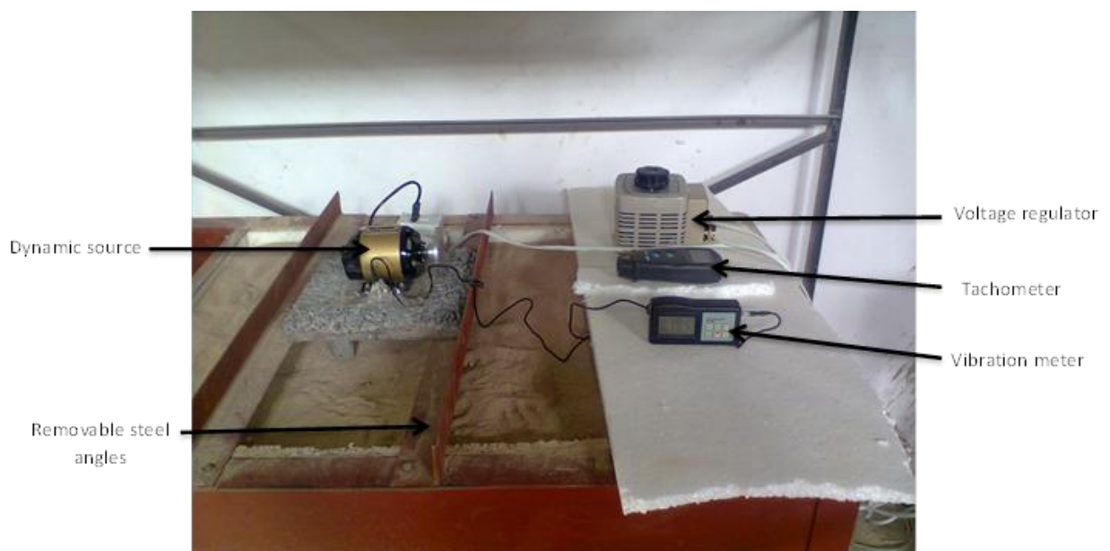
Figure (6) The Overall System
