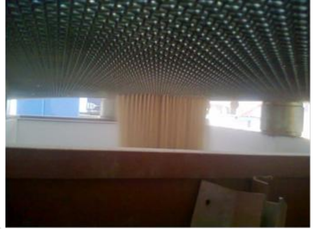
Figure (5) Raining Method to Control the Dry Density of Sand
