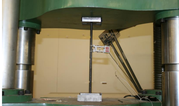
Figure 7: Monotonic tensile test setup
