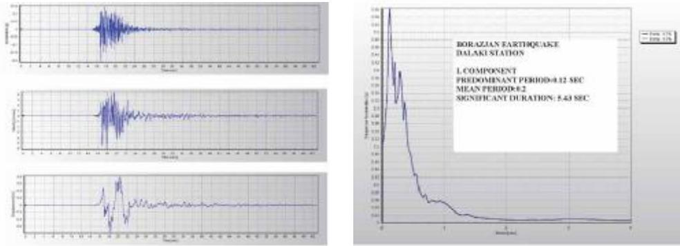
Figure 3. Acceleration, velocity, and displacement time histories of the transversal component recorded at Dalaki station (left), and response spectra of the same accelerogram (right).
