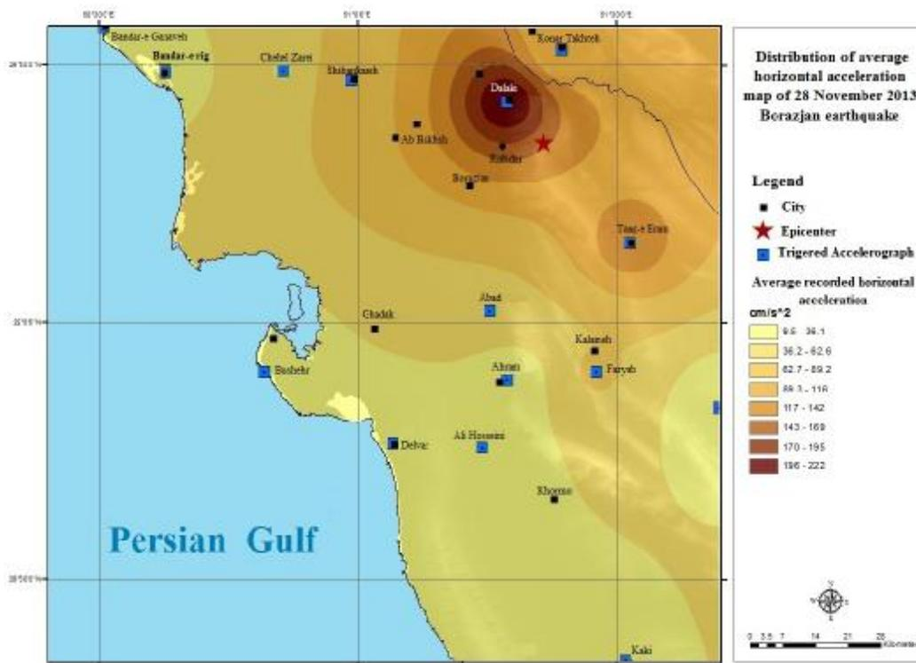
Figure 2. Distribution of average horizontal acceleration map based on the recorded accelerations in the earthquake stricken area.
