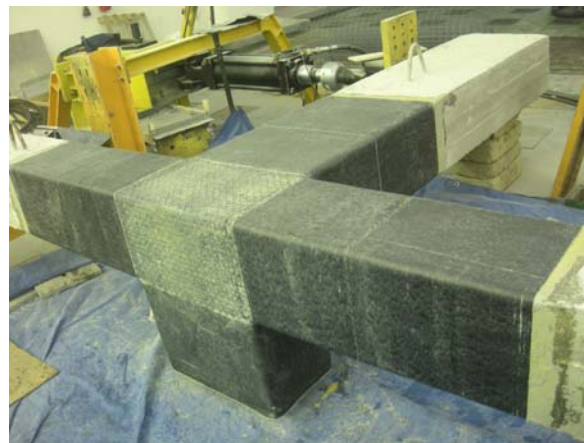
Figure 1. Experimental test on beam-column joints strengthened with FRP systems (Del Vecchio et al. 2014).
