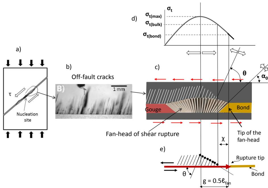
Figure 1. Explanation of features of the off-fault cracking process observed in the photoelastic experiments
