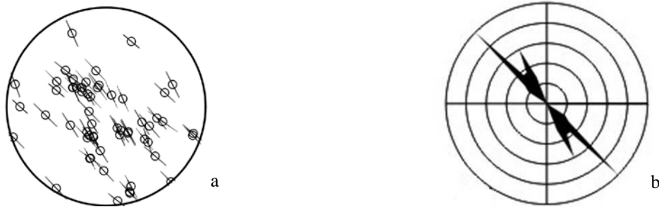
Figure 5. VIL2 station: (a) Polar equal-area projections on the upper hemisphere of the fast shear wave polarizations. The length of the bars is proportional to the time delay of each event and the circle represents an angle of incidence equal to 45^\circ . (b) Rose diagram of the fast shear wave polarization directions.
