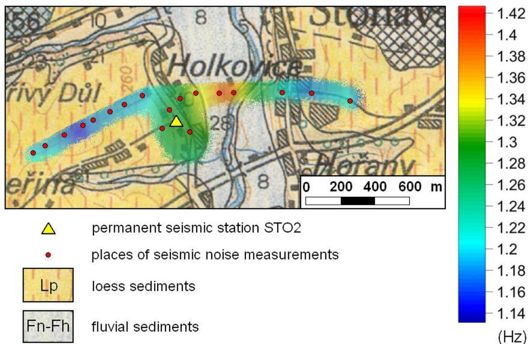
Figure 1. Geological map of Stonava village in the Karviná region with results of resonance frequency of sedimentary layers along the measured profile (tonality represents determined values)
