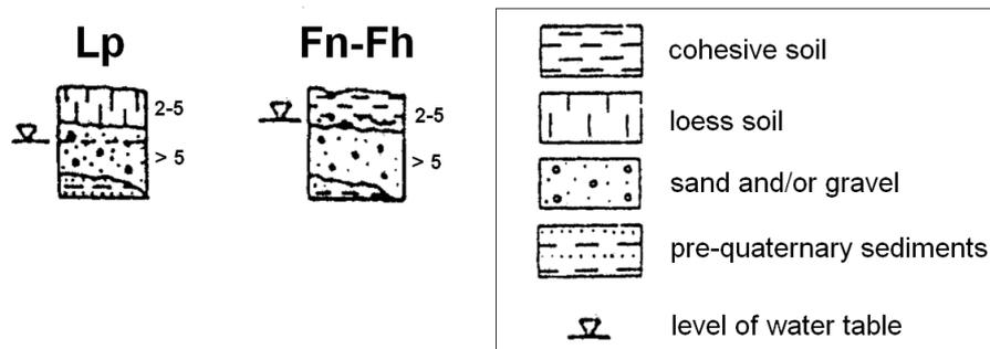
Figure 2. Example of the sections of sub-zones in Stonava locality with the thickness of Quaternary soils and with the average depth of groundwater table according the map of engineering geological zoning (Kašpárek 1998)
