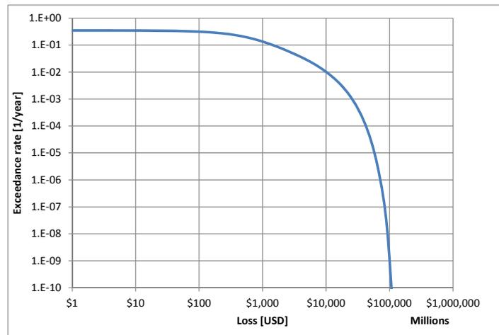
Figure 1. Seismic LEC for Medellin
