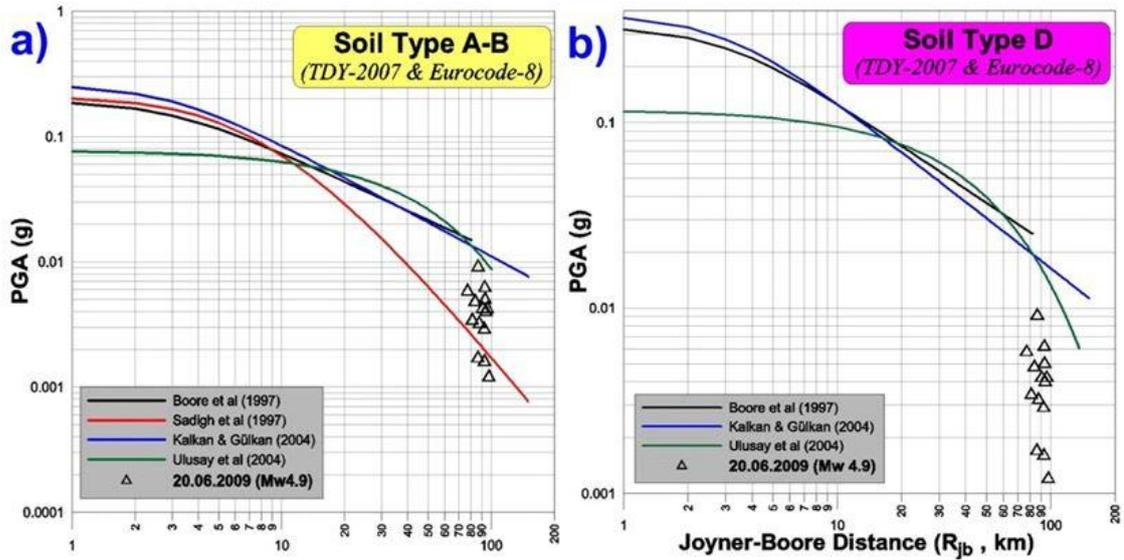
Figure 1. Excel otomatization for different type of attenuation relationship after a magnitude Mw=4.9 occurred in a distance ~90 km far on June 20, 2009. A) Attenuation distribution with distance was shown according to Turkish Earthquake Code (TDY) and Eurocode-8 for; a) soil type A&B, and b) soil type D.
