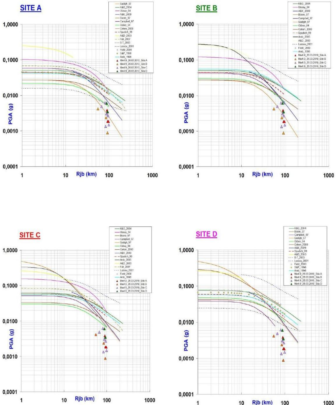
Figure 3: Different type of attenuation relationships after for Foca earthquake occurred in a distance between 50 and 100 km far with a magnitude  $M_w=5.3$  ( $M_L=5.0$ ) on May 1, 2012. Attenuation distribution was shown according to Turkish Earthquake Code (TDY) for soil types A, B, C and D (earthquake parameters are taken from AFAD Ankara). Triangles show measured peak acceleration values observed in different sites.
