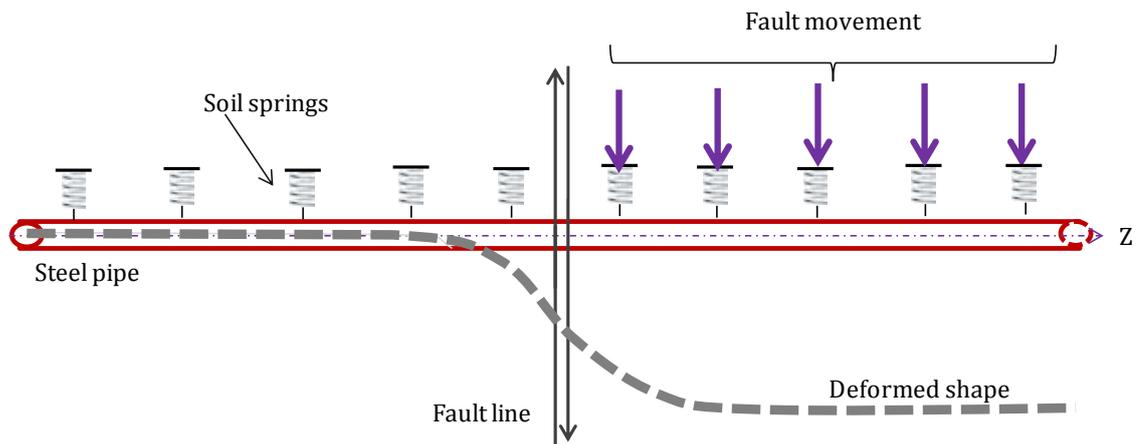
Figure 1. A plan view of the simple model representing pipe behavior under prescribed fault movement perpendicular to the pipe axis (Z axis)
