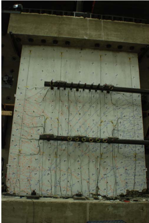
a) Modern slender wall test specimen (PW4) at the end of laboratory testing; compression failure of right boundary element resulted in loss of lateral strength
