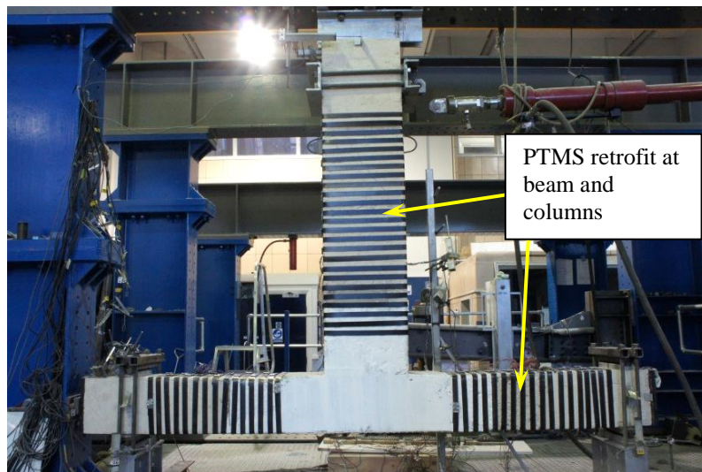
Figure 1. Retrofitting of beam and column of RC joint using the PTMS technique (column shown horizontally)
