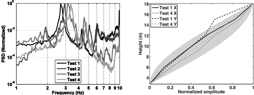
Figure 2. PSD spectra of recordings at the top of the structure throughout its retrofit (left). The increase of the resonance frequency with time is clear to be noticed. Modal shapes in elevation before (test 1) and after (test 4) retrofit. The grey shaded area delimits the range between the pure shear beam (lowest limit) and the cantilever beam (upper limit). The observed modal shapes behave more in shear after the retrofit due to the RC slabs.
