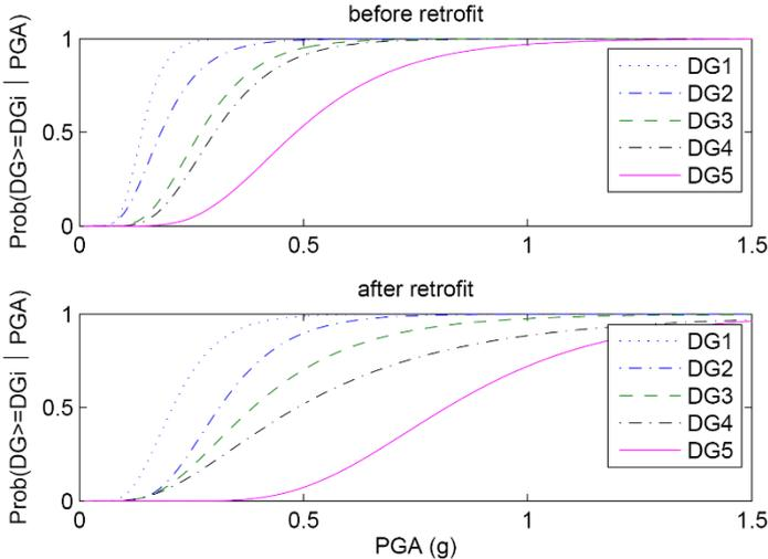
Figure 3. Fragility curves for the study-building before and after the retrofit
