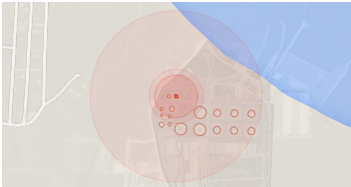
Figure 1. End-point distances for an earthquake-triggered pool fire at storage tank T2.
