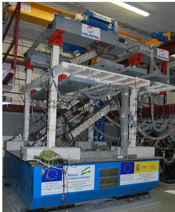
Fig. 3: Overall view of the shaking table test
